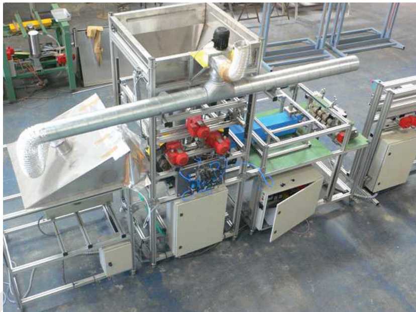
FIGURE 2. General overview of the powder coating equipment.
