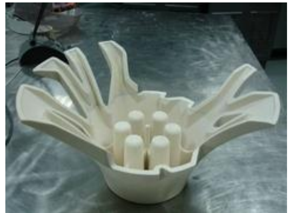
Figure 5 – Master being assembled in parts
