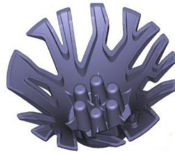
Figure 4 – Design of the master
