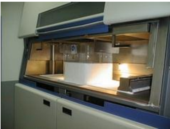
Figure 1 – Technology used to produce the master (Sinterstation 2500 from 3D Systems)
