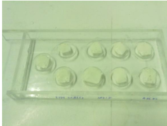
Figure 2.1 - Plate where the scales were glued and covered with silicon to form the molds with scale patterning
