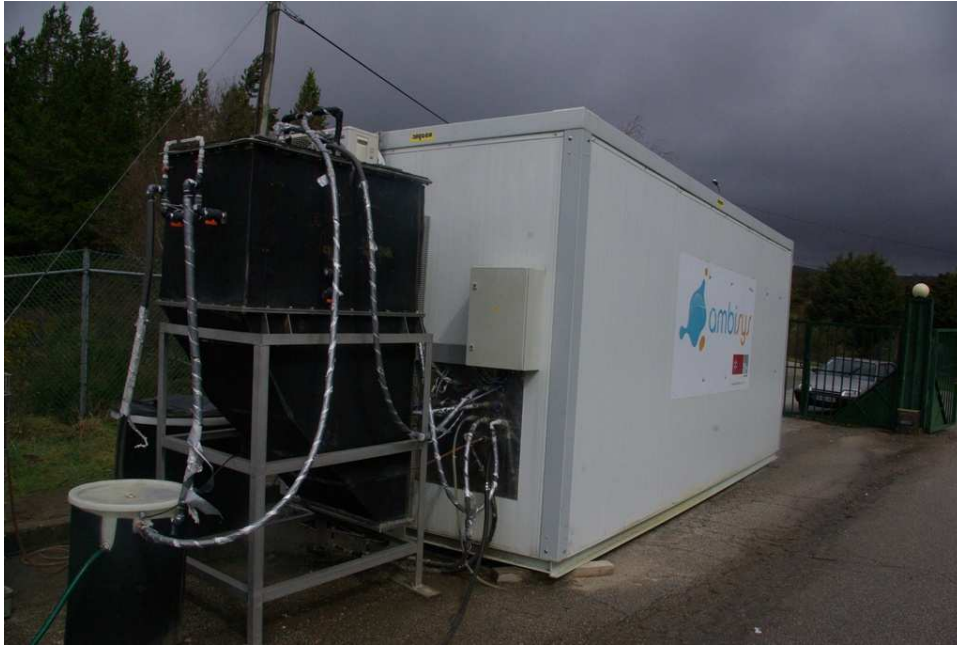
Figure 4.3 Mobile pilot plant including reactor in the forefront.
