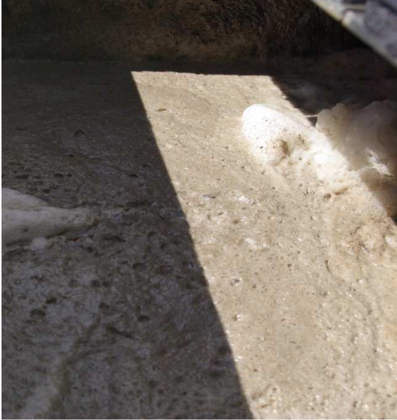
Figure 4.19 Floating layer in the top section of the reactor after addition of raw fat.
