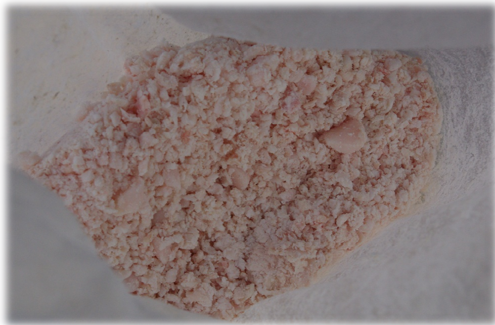
Figure 4.8 Photograph of the grated fat before addition to the reactor.
