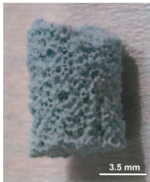
Figure 2. Macroscopic appearance of the HA scaffolds after sintering at 1300^\circ\text{C} . [Color figure can be viewed in the online issue, which is available at www.interscience.wiley.com .]
