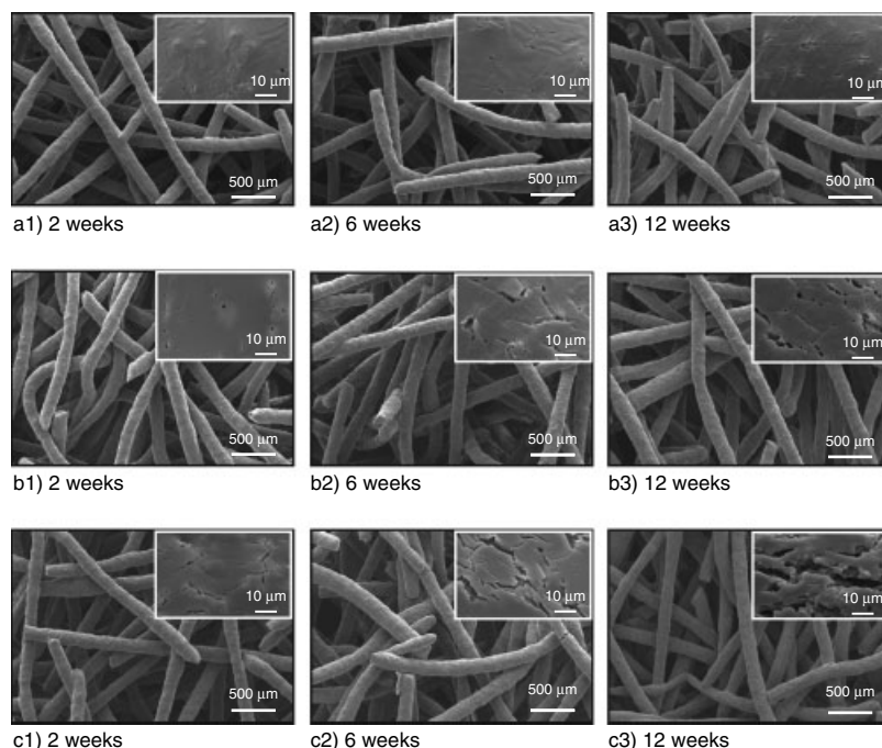
Figure 6. SEM micrographs of SPLA fiber meshes after degradation tests for different periods of time: a1) to a3) in PBS; b1) to b3) in PBS + \alpha -amylase solution; c1) to c2) in PBS + \alpha -amylase and lipase solution. Inserts correspond to magnifications of the respective pictures showing in detail the surface morphology of the degraded fibres
