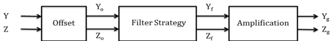
Figure 4.6 Diagram of the processing architecture of the Y and Z-signals.
