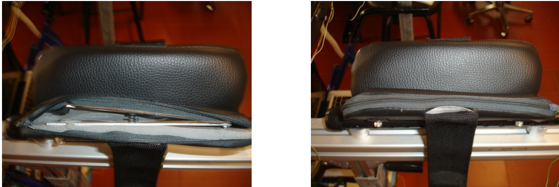
Figure 5.10 Assembly of the FlexiForce sensor with the forearm support.
