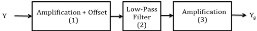
Figure 4.25 Diagram of the circuit hardware for the processing of the Y-signal.
