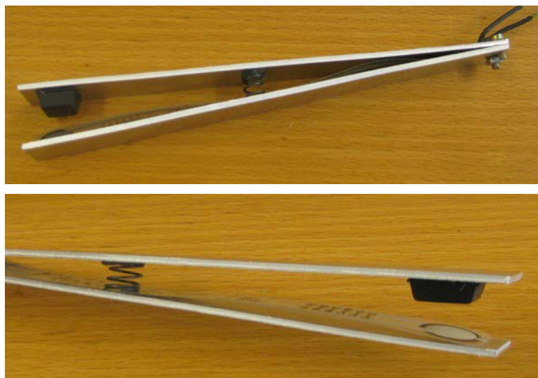
Figure 5.9 Mechanical device to support the sensor and ensure that the load made by the user on the forearm support is entirely made on the sensing area of the Flexiforce sensor.
