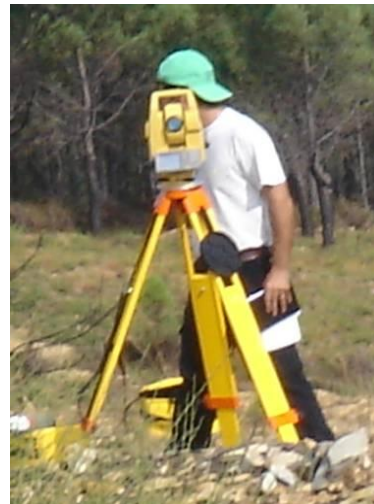
Photo 4. Survey of the plots and the study area with a total station
