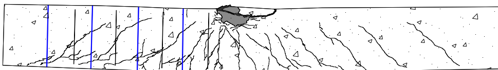
Figure 4.41 – Crack pattern at the end of the tested S225.90/E225.90 beam (Dalfré et al. 2011).
