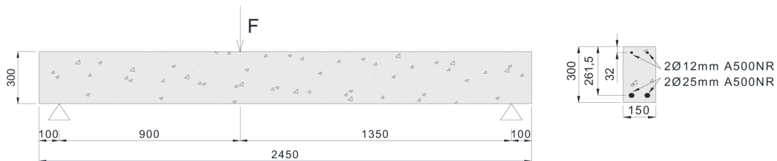
Figure 4.36 – Reinforced concrete beam: geometry, support, steel reinforcement scheme and loading conditions [dimensions in mm] (Dalfré et al. 2011).
