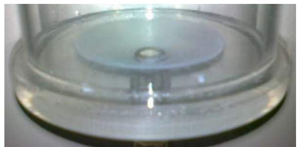
Fig 3: Filtration column detail: bottom retention structure
