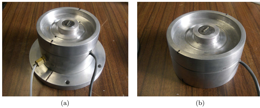
Figure 4.3: (a) Bottom and (b) top platens with embedded bender–elements (Ferreira et al. , 2010)
