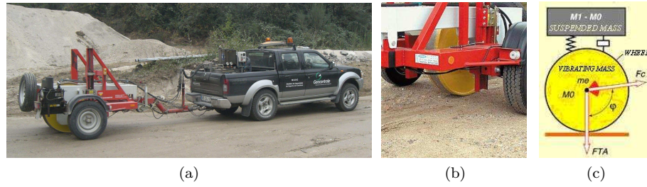
Figure 2.27: Portancemètre equipment: (a) general aspect; (b) vibrating wheel detail; (c) function schema
