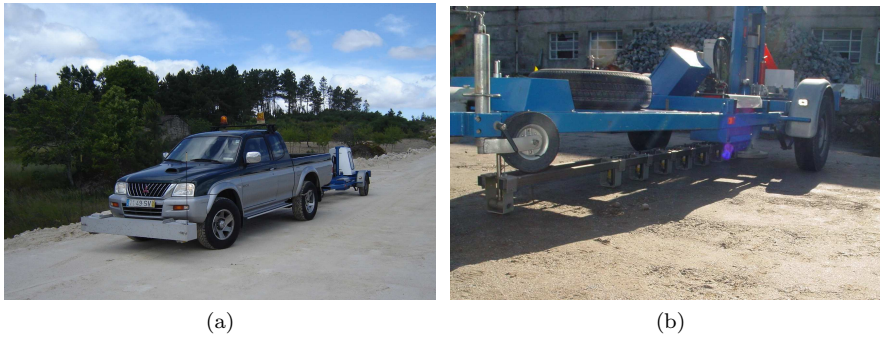
Figure 2.19: FWD : (a) general view; (b) detail of geophones and plate
