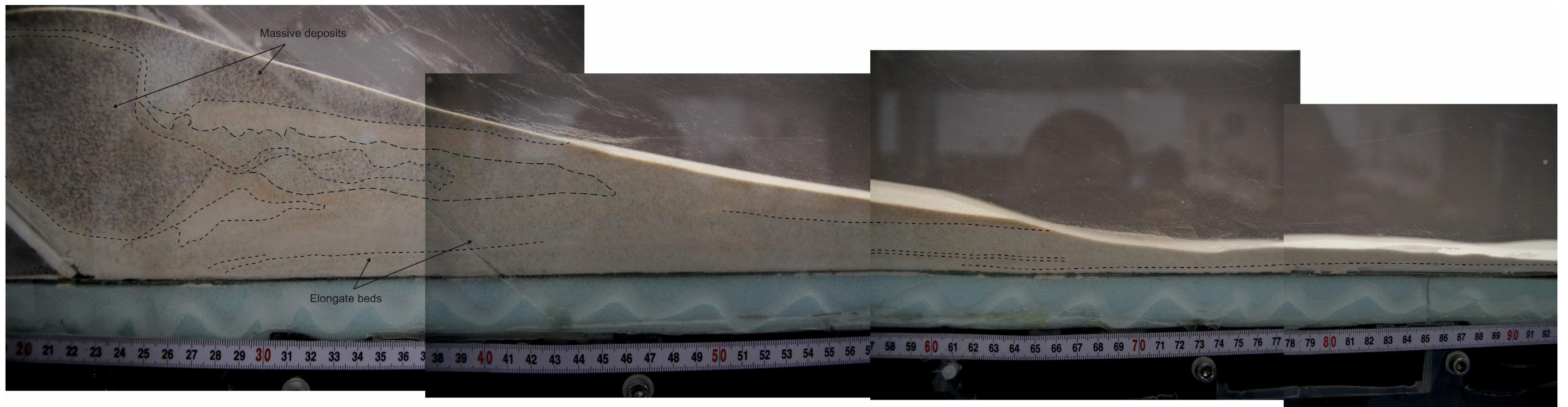
Figure 5.10: Annotated photograph of the deposit from the quad-disperse current showing an ungraded massive deposit of coarse material
