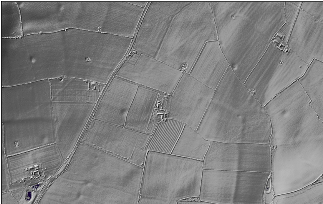
Figure three: An example of a topographical LIDAR image. This example clearly shows subtle marks in the earth's surface. This allows archaeologists to determine whether a place is archaeologically significant - grid reference SP3571662340 (Houseprices.io lab, 2019)
