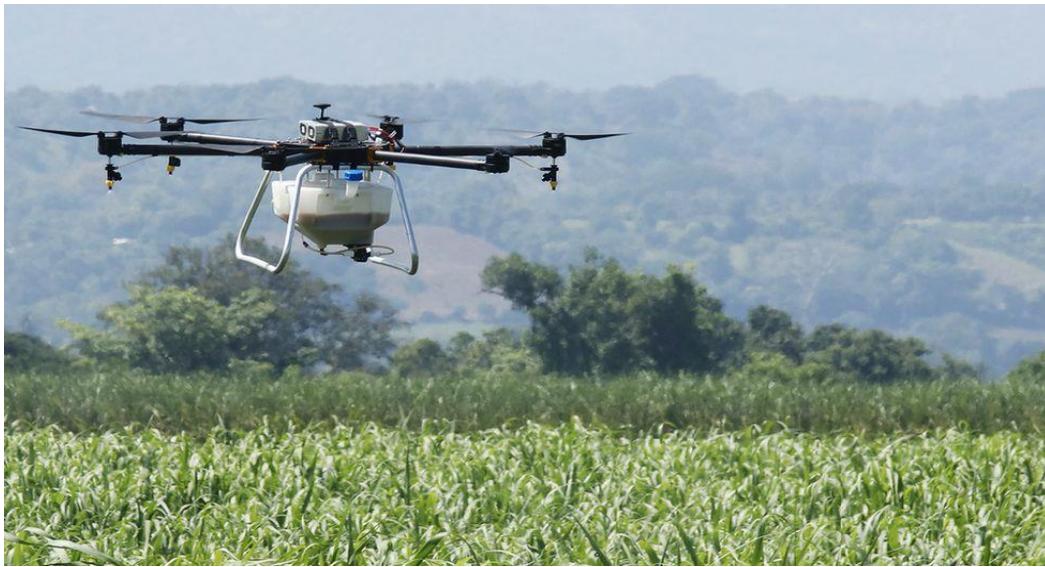
Figure 5.7 UAV used for spraying crops from (Baraniuk, 2018).
