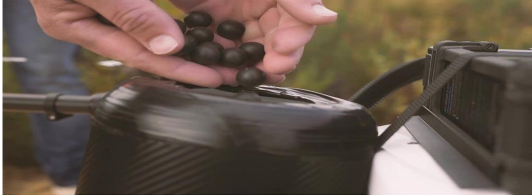
Figure 5.9 UAV and seed storage from (Caboz, 2019).
