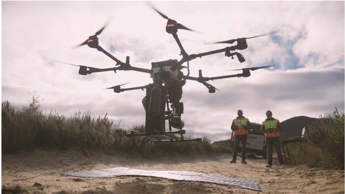
Figure 5.8 UAV used for planting trees from (Caboz, 2019).
