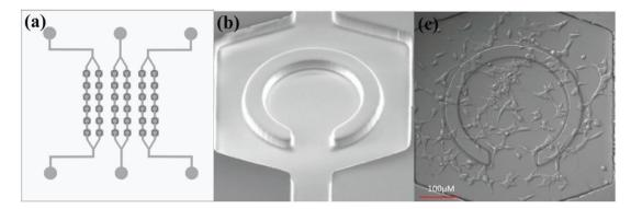
Figure 1.44: Chip design and cell culture. (a) Schematic illustration of the microfluidic channels with cell culture chambers. (b) A cell culture chamber with a C-shaped dam. (c) HEK293 cells cultured in a cell culture chamber.<sup>334</sup>
