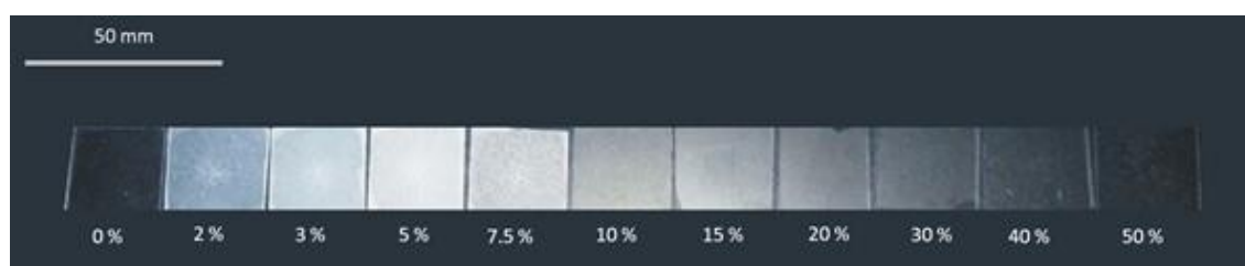
Figure 4.5 Digital photographs showing physical appearances of the different impregnated coatings fabricated with different concentrations of squalane in 5% fumed silica dispersion in ethanol. The coated slides are placed on a table with black background. The coatings obtained at both 0 and 50% squalane concentration are highly transparent as the colour of the table can be seen through the slides whereas the rest show different degree of opacity with a maximum at 5% squalane concentration.
