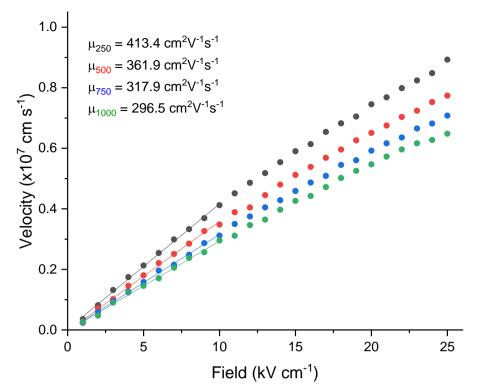
**Figure 4.3.1:** Linear fit analysis, performed within the OriginPro software, of the low-field steady state velocity vs field results, generating the electron mobility for each confining field strength. Colour and number in subscript corresponds to the colour of the data plot and confining field strength in kVcm<sup>-1</sup>.
