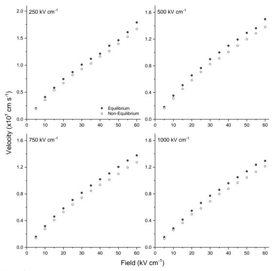
**Figure 5.1.3:** Average electron velocity vs applied electric field for confining fields ranging from 250-1000 kVcm<sup>-1</sup>, comparing the equilibrium results, from figure 4.1.1, (solid circles) to non-equilibrium results (open circles).
