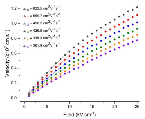
**Figure 4.5.2:** Linear fit analysis, performed within the OriginPro software, of the low-field steady state velocity results, generating the electron mobility for each alloy disorder potential. Colour and number in subscript corresponds to the colour of the data plot and alloy disorder potential in eV.
