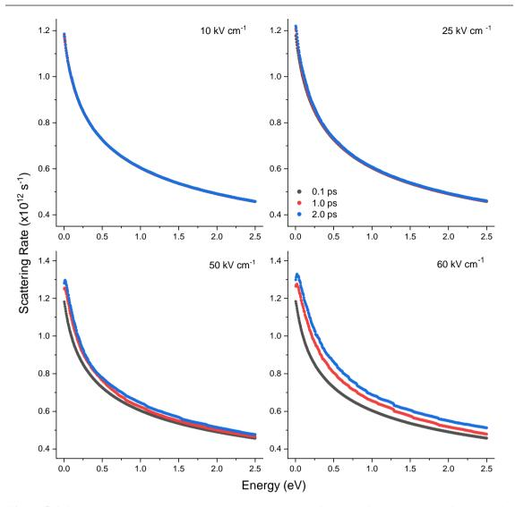
**Figure 5.6.6:** Intra-band POP via absorption scattering rates as a function of electron energy for an applied field of 10, 25, 50 and 60 kVcm<sup>-1</sup> after 0.1, 1 and 2 ps.
