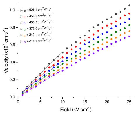
**Figure 5.5.2:** Linear fit analysis, performed within the OriginPro software, of the low-field steady state velocity results, generating the electron mobility for each alloy disorder potential. Colour and number in subscript corresponds to the colour of the data plot and alloy disorder potential in eV.
