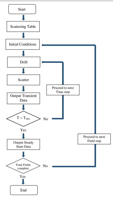
Figure 2.2.1: Flowchart showing an overview of how the base EMC algorithm simulates electron transport.
