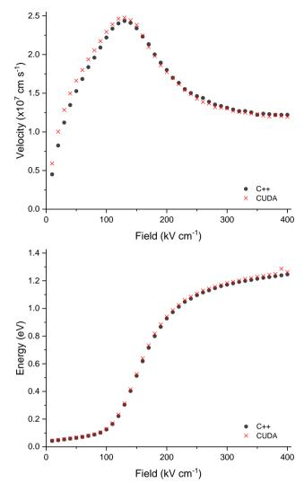
**Figure 3.2.3:** Steady state velocity and energy results, comparing results from the original C++ code (using doubles) to the CUDA code (using floats).
