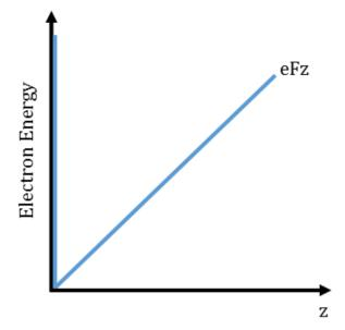
**Figure 2.3.1:** Illustration of the triangular potential well approximation of the conduction band, assuming the confinement is in the z-direction, for a confining electric field strength, F.
