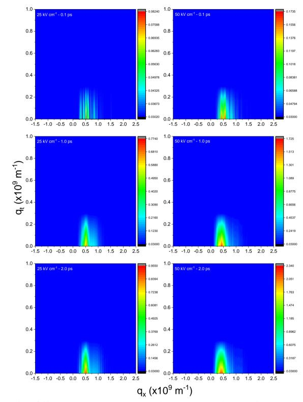
**Figure 5.6.2:** Phonon distributions as a function of phonon wavevector for applied fields of 25 and 50 kVcm<sup>-1</sup> after 0.1, 1 and 2 ps.  $q_x$  is the component of the phonon wavevector in the direction of the applied electric field (x-direction) and  $q_t$  is the y-z component. Confining field strength of 500 kVcm<sup>-1</sup>.
