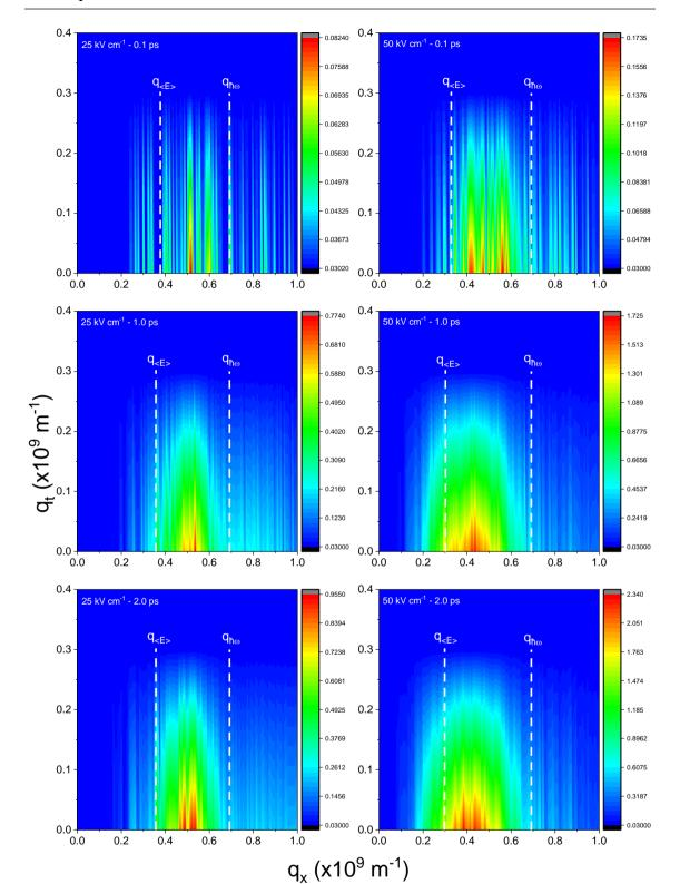
**Figure 5.6.3:** Phonon distributions as a function of phonon wavevector for an applied field of 25 and 50 kVcm<sup>-1</sup> after 0.1, 1 and 2 ps, for a confining field strength of 500 kVcm<sup>-1</sup>.  $q_{\hbar\omega}$  represents the minimum wavevector calculated from the minimum in-plane energy required to emit a phonon,  $q_{\langle E \rangle}$  represents the minimum wavevector calculated based on the average in-plane energy for the given snapshot.
