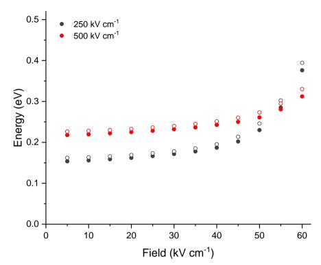
**Figure 5.1.1:** Average electron energy vs applied electric field for confining field strengths of 250 and 500 kVcm<sup>-1</sup>. Results from both the equilibrium, figure 4.1.3, (solid circles) and non-equilibrium (open circles) simulations are shown for comparison.
