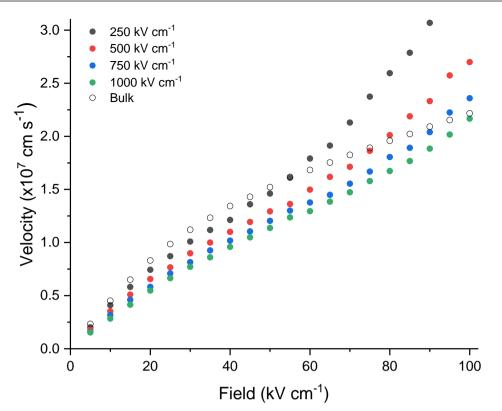
**Figure 4.1.1:** Average electron velocity vs applied electric field, confining fields from 250-1000 kVcm<sup>-1</sup>, compared to results from the bulk Monte Carlo.
