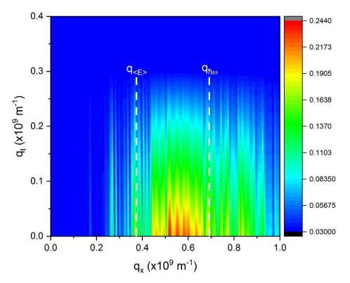
**Figure 5.6.5:** Phonon distribution as a function of phonon wavevector for an applied field of 10 kVcm<sup>-1</sup> after 2 ps, for a confining field strength of 500 kVcm<sup>-1</sup>.  $q_{\hbar\omega}$  represents the minimum wavevector calculated from the minimum in-plane energy required to emit a phonon,  $q_{\langle E \rangle}$  represents the minimum wavevector calculated based on the average in-plane energy for the given snapshot.
