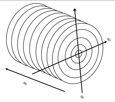
**Figure 2.4.2:** Schematic diagram showing the q-space grid, consisting of concentric circles, centred along the  $q_x$  axis and with increasing radii in the y-z plane.
