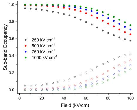
Figure 4.1.4: First sub-band (solid circles) and second sub-band (open circles) occupancy vs field for a range of confining fields.
