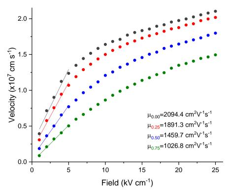
**Figure 4.5.3:** Linear fit analysis, performed within the OriginPro software, of the low-field steady state velocity results, generating the electron mobility for further reduced alloy disorder potential. Colour and number in subscript corresponds to the colour of the data plot and alloy disorder potential in eV.
