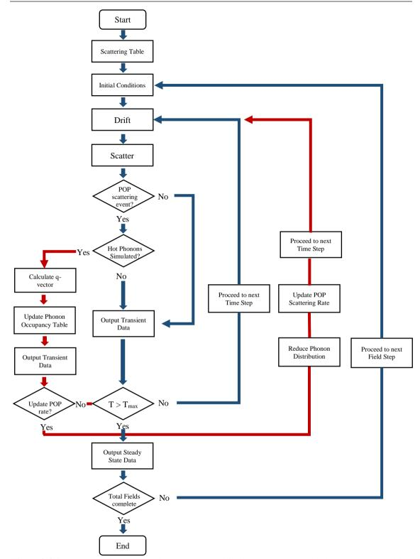
Figure 2.4.1: Flowchart diagram showing how non-equilibrium phonons are added to an EMC algorithm.
