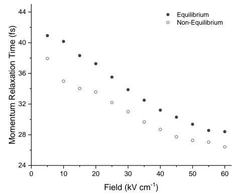
**Figure 5.2.1:** Momentum relaxation time vs applied electric field for a confining field of 500 kVcm<sup>-1</sup>, comparing equilibrium (solid circles) and non-equilibrium (open circles) results.
