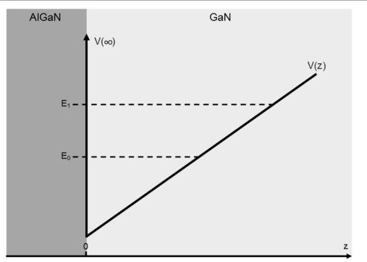
**Figure 4.1:** Schematic diagram of a triangular potential well at an AlGaN/GaN interface.  $E_0$  and  $E_1$  represent the sub-band energy levels,  $V(\infty)$  represents the infinite potential assumed at the interface (z=0), V(z) is the potential as a function of z, i.e. the depth into the GaN layer.
