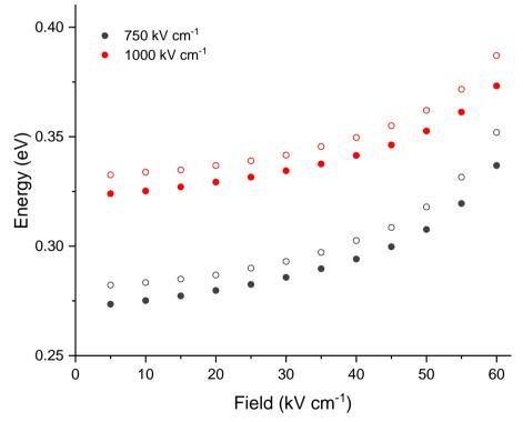
**Figure 5.1.2:** Average electron energy vs applied electric field for confining field strengths of 750 and 1000 kVcm<sup>-1</sup>. Showing results for equilibrium, figure 4.1.3, (solid circles) and non-equilibrium (open circles) simulations for comparison.
