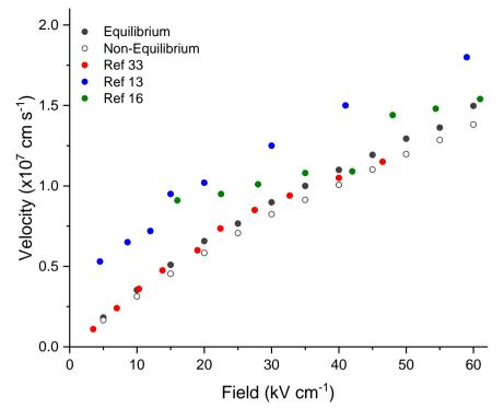
**Figure 5.1.4:** Average electron velocity vs applied electric field results from the equilibrium and nonequilibrium 2DEG simulations (confining field of 500 kV cm<sup>-1</sup>, alloy disorder potential of 1.5 eV), compared to simulation results from Palacios [33], and experimental results from Matulionis for a 3 ns [13] and 100 ns voltage pulse [16].
