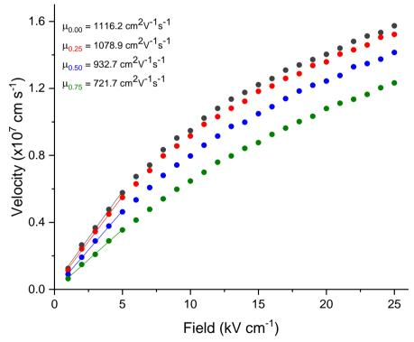
**Figure 5.5.3:** Linear fit analysis, performed within the OriginPro software, of the low-field steady state velocity results, generating the electron mobility for further reduced alloy disorder potential. Colour and number in subscript corresponds to the colour of the data plot and alloy disorder potential in eV.
