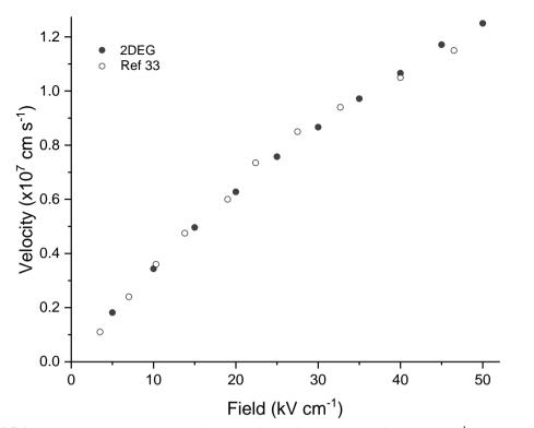
**Figure 4.5.4:** Steady state velocity results for a confining field strength of 8400 kVcm<sup>-1</sup> (corresponding to an electron sheet density of 1.46x10<sup>13</sup> cm<sup>-2</sup>) and an alloy disorder potential of 0.9 eV, compared to experimental results from Palacios [33].
