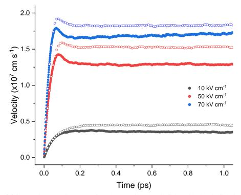
**Figure 4.4.1:** Transient velocity results for a low applied electric field, mid-electric field just before the energy runaway, and just after the energy runaway in the 2DEG (solid circles) and corresponding data from the bulk EMC (open circles).
