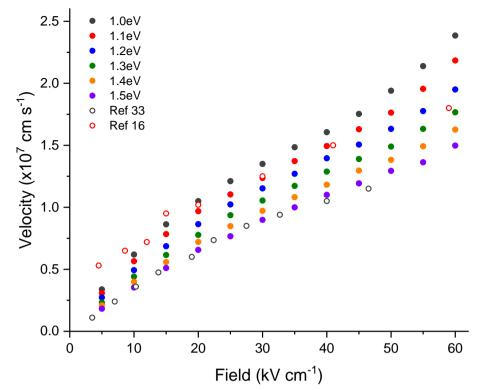
**Figure 4.5.1:** Steady state velocity results for varying alloy disorder potential, compared to experimental results from Palacios [33] and Matulionis [16].
