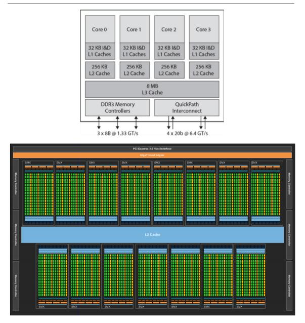
**Figure 1.3.1:** Illustration of the CPU and GPU architectures, showing the vast difference in cores. The CPU diagram (top) is based on the Intel Core processors, and the GPU diagram (bottom) is the block diagram of a NVIDIA Kepler GK110, where each green or yellow block represents a CUDA core [52].
