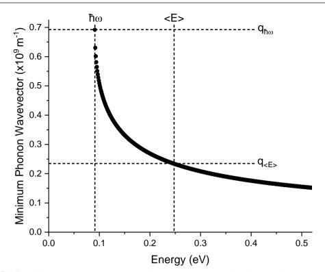
**Figure 5.6.4:** Minimum phonon wavevector against electron energy. Showing the phonon energy,  $\hbar\omega$ , the ensemble average energy (taken at 0.1 ps for an applied electric field of 50 kVcm<sup>-1</sup>), <E>, and the associated minimum phonon wavevectors for each energy.
