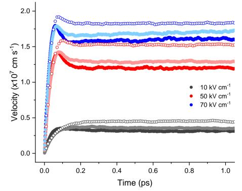
**Figure 5.4.1:** Transient velocity characteristics for a low applied electric field, mid-electric field before the energy runaway and just after the energy runaway (in equilibrium). Comparing the equilibrium 2DEG (pale solid circles), non-equilibrium 2DEG (solid circles) and equilibrium bulk EMC (open circles) results.
