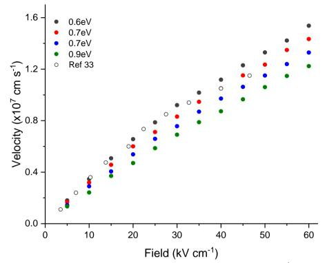
**Figure 5.5.4:** Steady state velocity results for a confining field strength of 8400 kVcm<sup>-1</sup> (corresponding to an electron sheet density of 1.46x10<sup>13</sup> cm<sup>-2</sup>) and alloy disorder potentials of 0.6, 0.7, 0.8 and 0.9 eV, compared to experimental results from Palacios [33].
