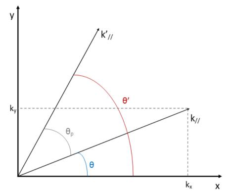
**Figure 2.3.2:** Illustration of the use of the Price scattering angle,  $\theta_p$ , and initial wavevector direction with respect to the x-axis,  $\theta$ , to generate the post-scatter angle between the final wavevector and the x-axis,  $\theta'$ . using the trigonometric functions  $\cos(A+B) = \cos(A)\cos(B) - \sin(A)\sin(B)$ , and  $\sin(A+B) = \sin(A)\cos(B) + \cos(A)\sin(B)$ . Using  $\theta$ ,  $\theta_p$  and  $\theta'$  from figure 2.3.2 this gives:
