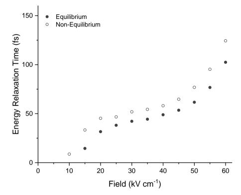
**Figure 5.2.2:** Energy relaxation time vs applied electric field for a confining field of 500 kVcm<sup>-1</sup>, comparing equilibrium (solid circles) and non-equilibrium (open circles) results.
