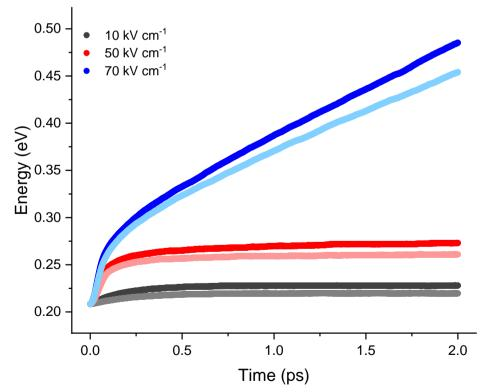
**Figure 5.4.2:** Transient energy characteristics for a low applied electric field, mid-electric field before the energy runaway and just after the energy runaway (in equilibrium). Comparing the non-equilibrium (solid circles) and equilibrium (pale solid circles) results.
