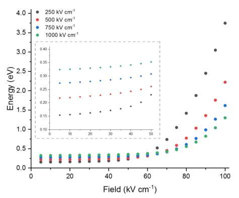
**Figure 4.1.3:** Steady state ensemble average total electron energy vs field plots for a range of confining electric fields, showing a rapid increase in electron energy at high fields. Subset shows the low field range.
