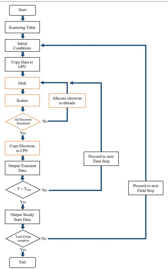
**Figure 3.2.1:** Flowchart showing an overview of how the base EMC algorithm was redesigned to run on a GPU. Orange borders represent sections performed on the GPU.
