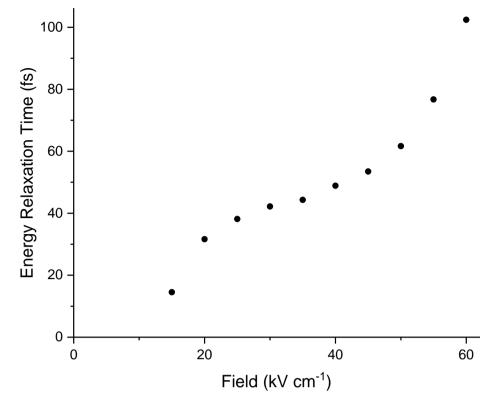
**Figure 4.2.2:** Energy relaxation times vs field, with a confining field of 500 kVcm<sup>-1</sup>, subset showing the low field range.
