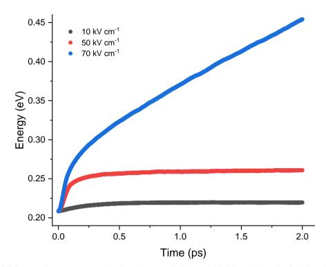
**Figure 4.4.2:** Transient energy results for a low applied electric field, mid-electric field just before the energy runaway, and just after the energy runaway in the 2DEG.
