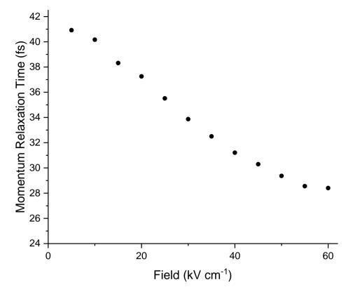
Figure 4.2.1: Momentum relaxation times vs field, with a confining field of 500 kVcm<sup>-1</sup>.
