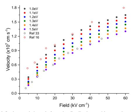
**Figure 5.5.1:** Steady state velocity results for varying alloy disorder potential, compared to experimental results from Palacios [33] and Matulionis [16].
