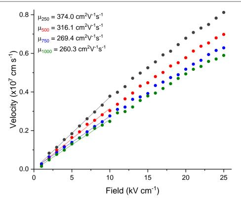
**Figure 5.3.1:** Linear fit analysis, performed within OriginPro, of the non-equilibrium low-field steady state velocity-field results, generating the electron mobility for each confining field strength. Colour and number in subscript corresponds to the colour of the data plot and confining field strength in kVcm<sup>-1</sup>.
