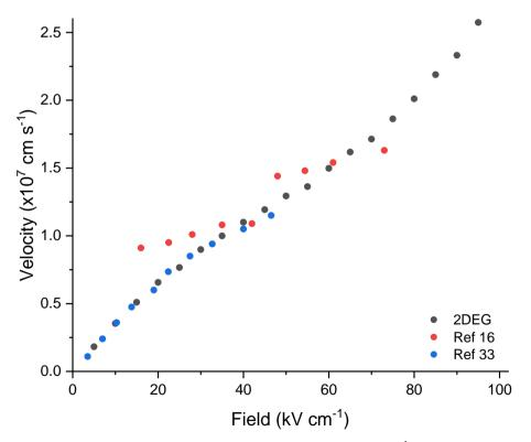
**Figure 4.1.2:** Average electron velocity vs field for the 2DEG (500 kVcm<sup>-1</sup> confining field), compared to experimental results from Matulionis [16] and Palacios [33].
