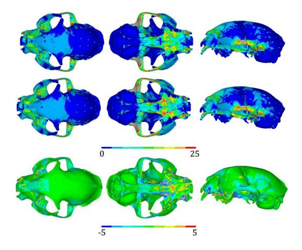
Figure 6.5. von Mises stress analyses (bilateral canine biting regime) for the nasal septum. Top row: model with nasal septum. Middle row: model without nasal septum. Bottom row: difference plots.
