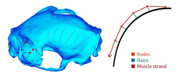
Figure 4.8. Left: Final distribution of the link elements (dark blue) over the cat's cranium model representing the superficial temporalis. Right: schematic drawing of the muscle wrapping solution representing the hairs and nodes of a single muscle strand in frontal view.
