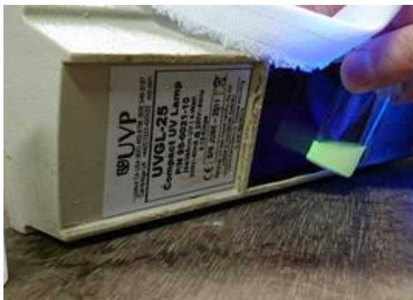
Figure 121. Image taken showing the fluorescence of fluorescamine in the presence of primary amines on the surface of nanoparticles [50].
