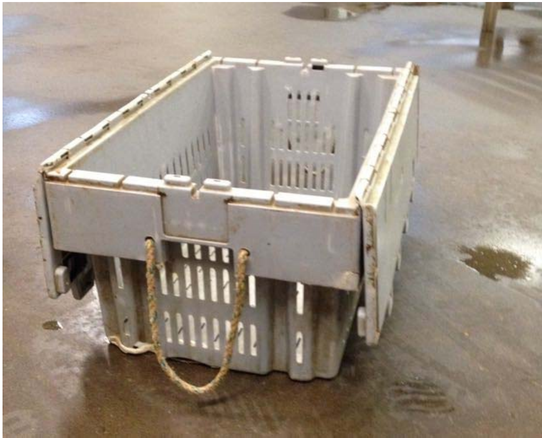
Figure 1.8 Vented plastic lobster crate in common use in the post-harvest transport and short-term storage of the Homarus americanus fishery.
