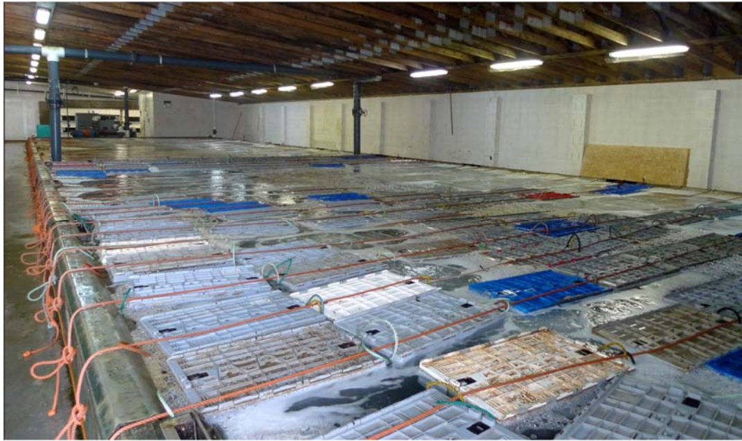
Figure 2.4 Typical Homarus americanus lobster crate reception reservoir used to immerse 40kg capacity lobster crates for recovery or short-term storage. Clearwater Seafoods, Clark's Harbour, Nova Scotia.
