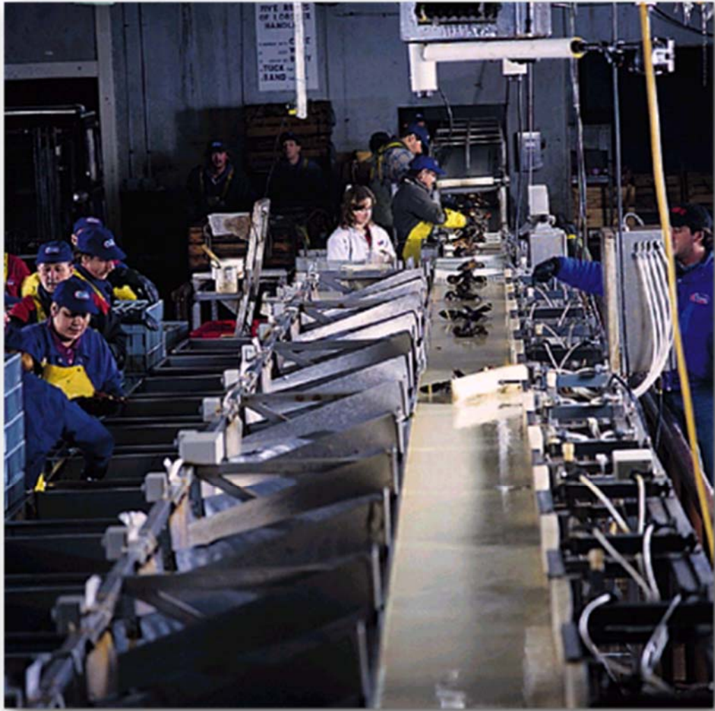
Figure 1.11 Homarus americanus live lobster automatic size and quality grading line system (from Clearwater Seafoods)
