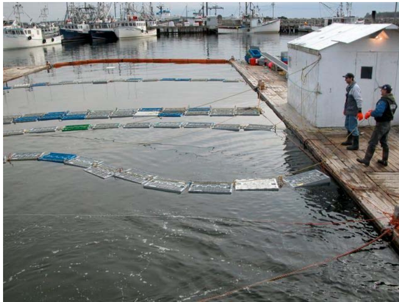
Figure 1.9 Typical shore-side reception temporary storage system in the Homarus americanus fishery. This photo shows a version with supplemental aeration. Crates are strung together with nylon rope (Clearwater Seafoods LP Photo).
