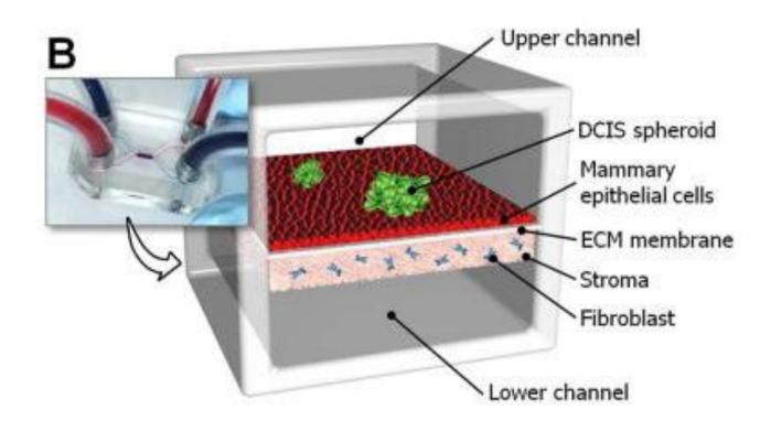
Figure 1.4: Microfluidic device for mimicking early stage breast cancer taken from (Choi et
