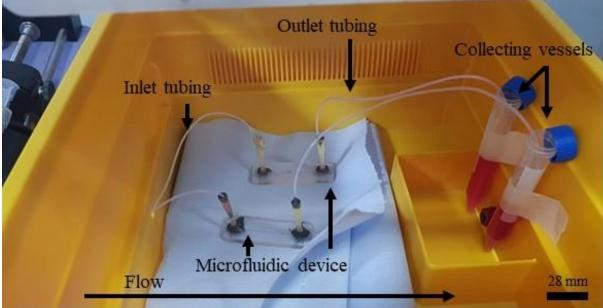
Figure 2.8: Egg incubator and microfluidic device set up
