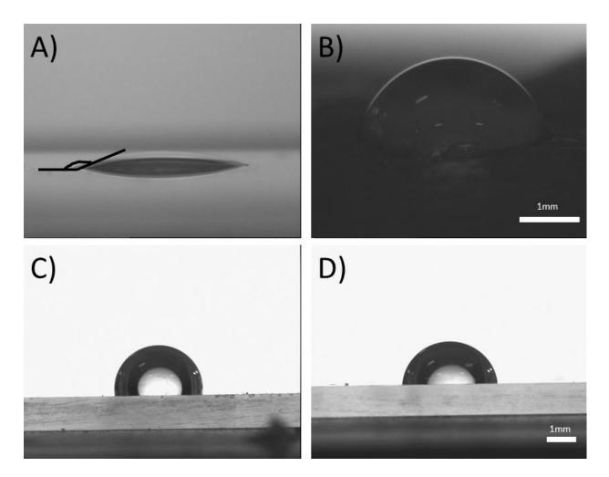
Figure 5.2: Representative images of water droplets used to measure contact angles on microscope slides after various surface treatments
