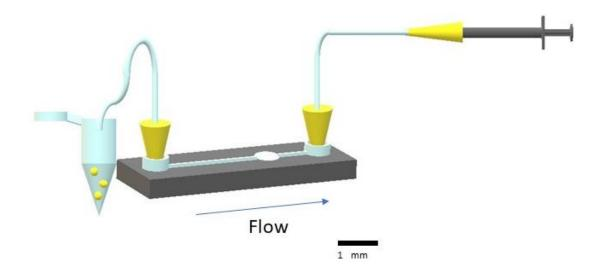
Figure 2.7: Setup used for the placement of spheroids into microfluidic device.
