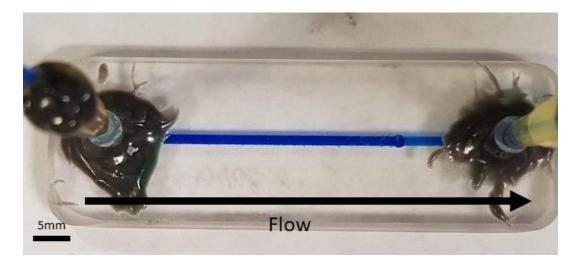
Figure 4.1: Generation 1 microfluidic device design
