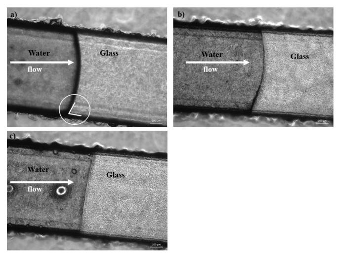
Figure 5.4: Representative images of water flowing within the microfluidic device microchannels. The water and glass angle was used to measure contact angles to prove surface treatments
