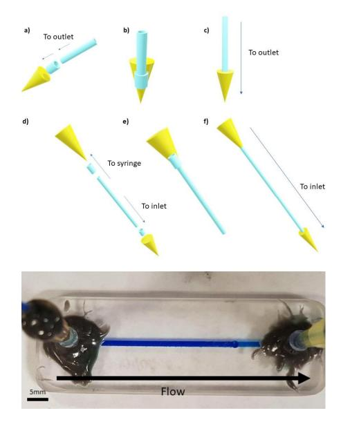
Figure 2.6: Generation 1 inlet and outlet tubing and the microfluidic device image
