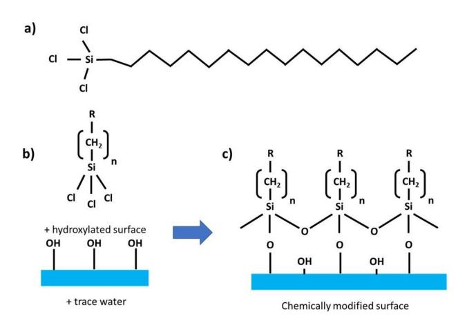
Figure 2.9: Octadecyltrichlorosilane chemical structure and glass surface modification
