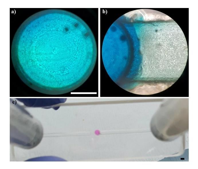
Figure 5.17: Successful hydrogel incorporation within a generation 3 microfluidic device
