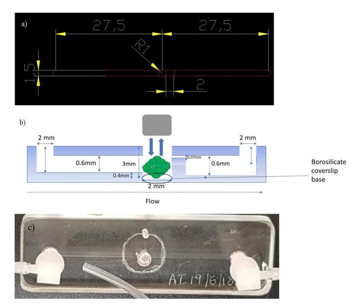
Figure 5.13: Generation 3 microfluidic device panel image (schematic and cross sectional)
