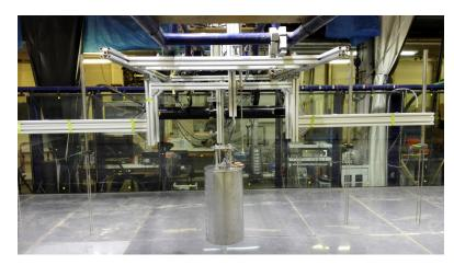
FIGURE 1.9: Close-up of the 1/50 scale PAWEC designed at University of Hull
