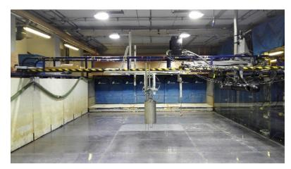
FIGURE 1.8: 1/50 scaled PAWEC and corresponding experimental wave tank at UoH (Jin et al., 2018).
