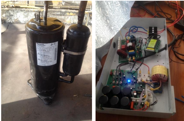
Fig. 4- 2: Image of the inverter compressor and frequency converter
