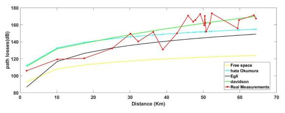
Figure 5-12: Propagation Models without Terrain
