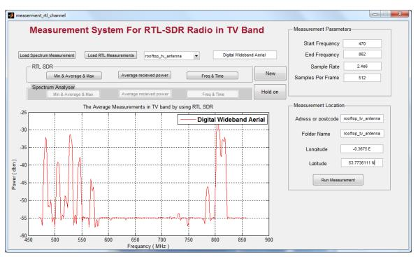
Figure 4-11: The GUI for the RTL-SDR System
