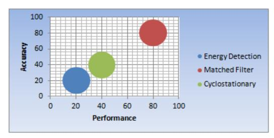
Figure 3-6: Comparison of spectrum sensing techniques (Singh, 2012a)
