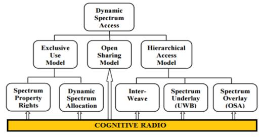
Figure 2-1: Dynamic Spectrum Access models
