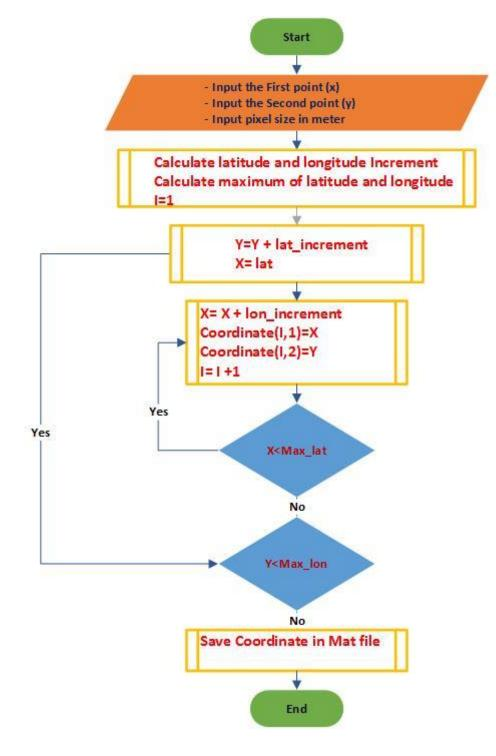
Figure 6-4: Algorithm of the Pixels Calculation
