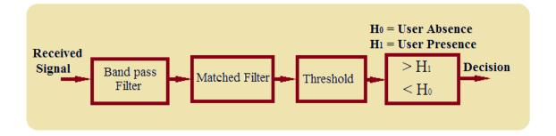
Figure 3-4: Matched Filter Detection block diagram
