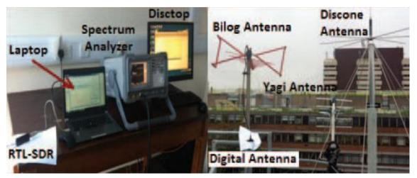
Figure 4-10: Measurement equipment in this paper: Antennas, spectrum analyser,
