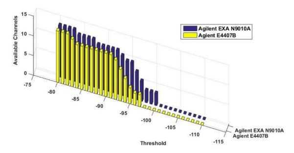
Figure 6-19: Calculate Thresholds, and Corresponding Available channels in both devices
