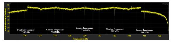
Figure 4-9: Channel 53 after combined the Measurement segments frequency range 726 MHz to 734 MHz
