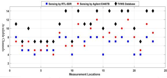
Figure 6-21: Comparison of combining techniques by using RTL-SDR and spectrum Analyser E4407B in different locations
