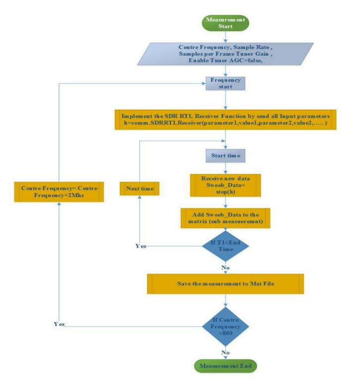
Figure 4-12: Signal calculation and Measurement methodology
