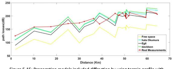
Figure 5-15: Propagation models included diffraction by using terrain profile with resolution 3 Arc second
