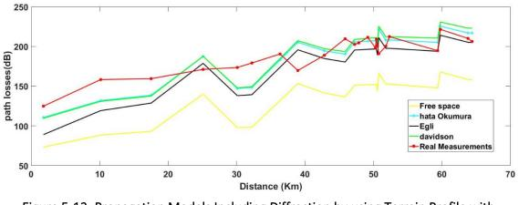
Figure 5-13: Propagation Models Including Diffraction by using Terrain Profile with Resolution 30 Arc Second (1 Km).
