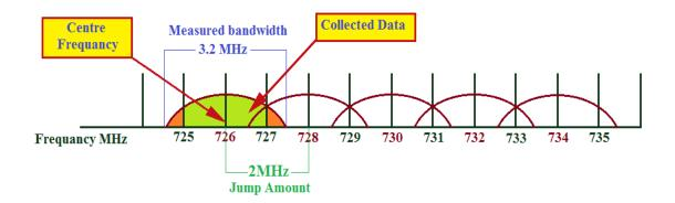
Figure 4-6: RTL-SDR Measurement Technique
