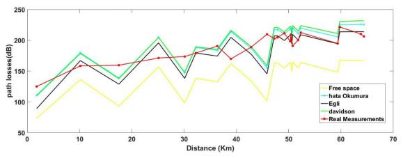
Figure 5-14: Propagation Models Included Diffraction by using Terrain Profile with Resolution 1 Arc Second
