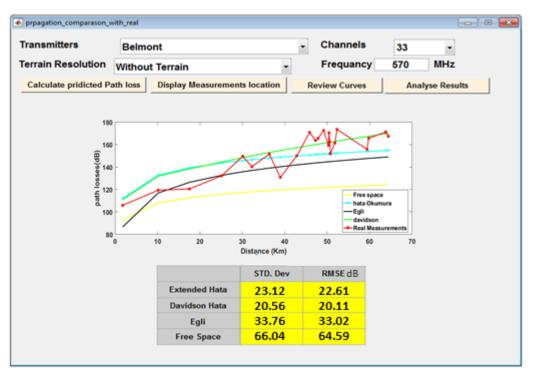
Figure 5-11: Example of propagation model comparison in the selected measurement locations
