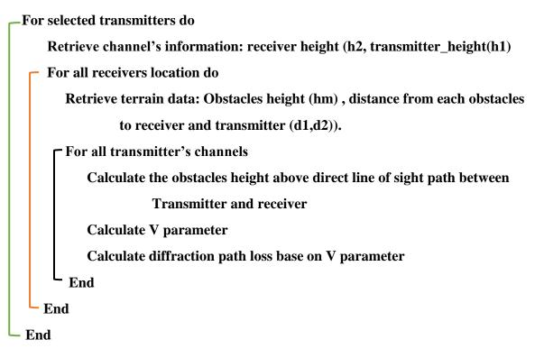
Figure 5-10: Algorithm of Diffraction Calculation
