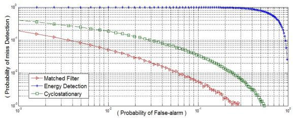
Figure 3-7: Complementary ROC curves for various spectrum sensing techniques (ED, MFD, CFD) with SNR=0 dB
