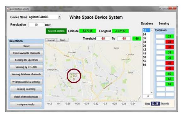
Figure 6-15: Results of combining techniques by using Agilent E4407B for sensing only database channels
