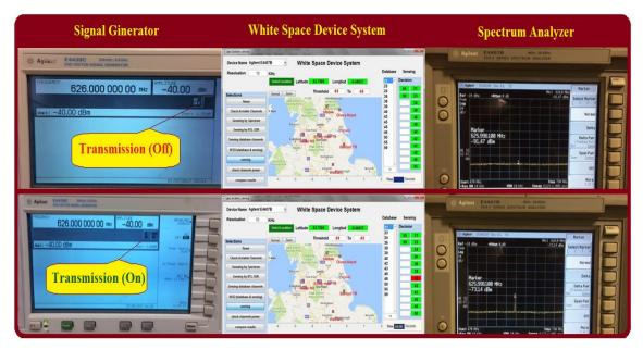
Figure 6-12: The white space system status before and after transmitting a test TV signal
