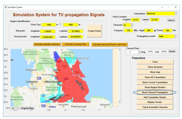
Figure 8.6: TV white space database system- Display channel propagation
