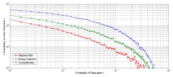
Figure 3-8: Complementary ROC curves for various spectrum sensing techniques (ED, MFD, CFD) with SNR=6 dB
