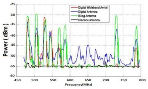
Figure 4-15: Average received power versus the frequency Band 470-862 MHz by using spectrum analyser.
