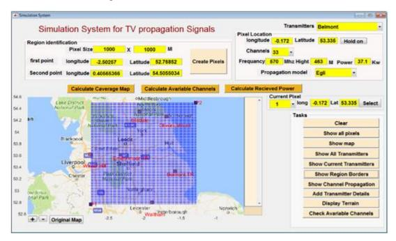
Figure 6-3: Display of all pixels in the selected region in the flexible simulation system for creating TVWS database
