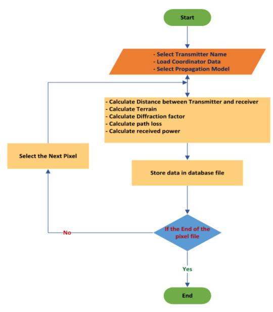
Figure 6-5 Algorithm of the received power calculation
