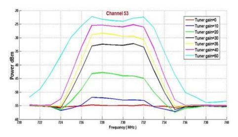
Figure 4-16: Average received power of channel 53 by different value of tuner gain
