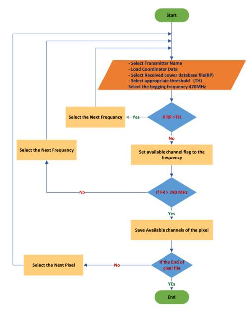
Figure 6-6 Available Channels Algorithm
