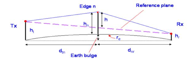
Figure 5-8: Path profile model for (single) knife edge diffraction.
