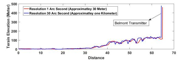
Figure 5-5: Terrain Elevation Data of path from university of Hull to Belmont Transmitter in different resolutions
