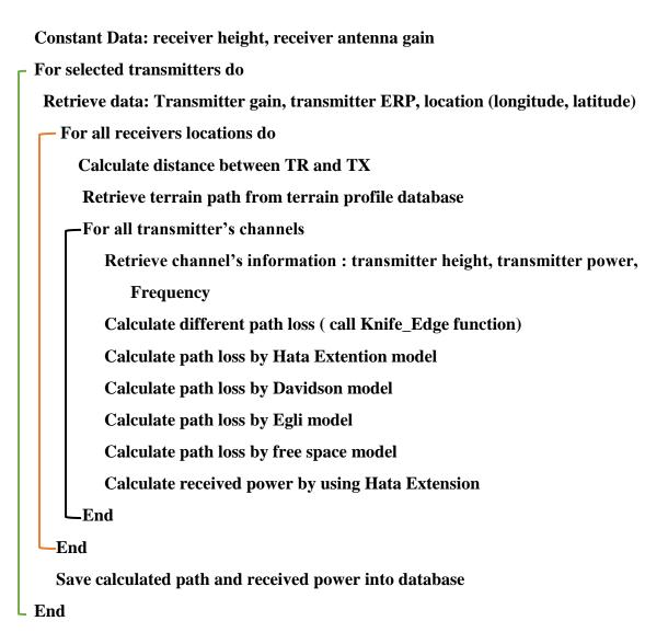
Figure 5-9: Algorithm of Propagation models Calculation.
