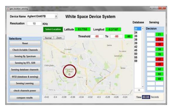
Figure 6-13: Result of combining techniques by using Agilent E4407B with threshold
