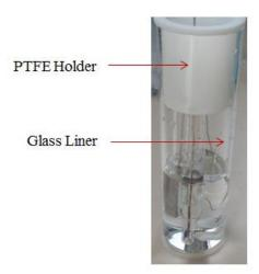
Figure 4.5 PTFE electrode holder inserted in the glass liner(100ml)
