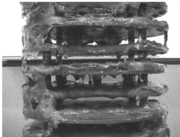
Figure 8. Photograph of the bottom plates of the first module showing the biofilm growth on the BPT plates. The huge biofilm does not endanger the permeability of the system.
