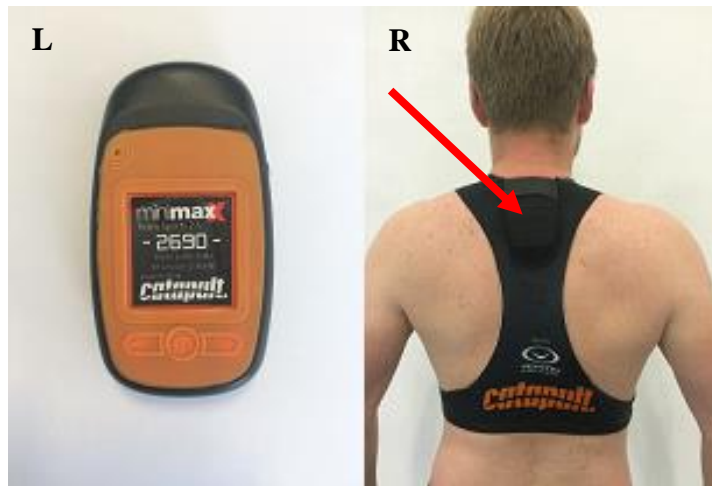
Figure 3.1. Portable MEMS device (L) and fast bowler wearing a bespoke neoprene vest (R). The arrow indicates unit placement, between the scapulae within a custom-made pouch as part of the bespoke neoprene vest.
