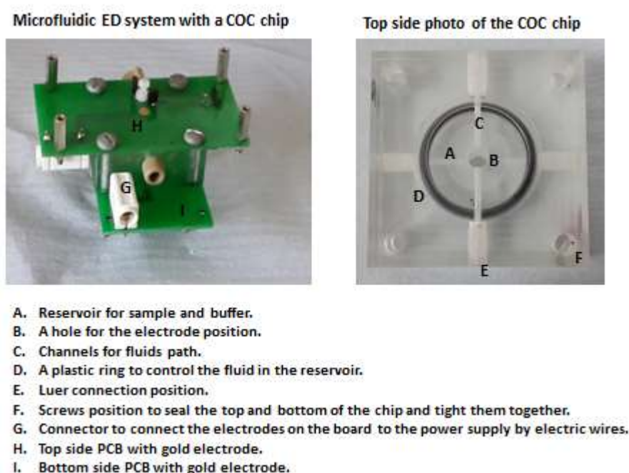
Figure 3-22: A photo of the ED system used for the extraction of ions
