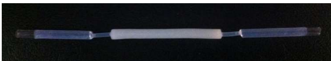
Figure 4-1: 6 cm long silica-based monolithic column for separation
