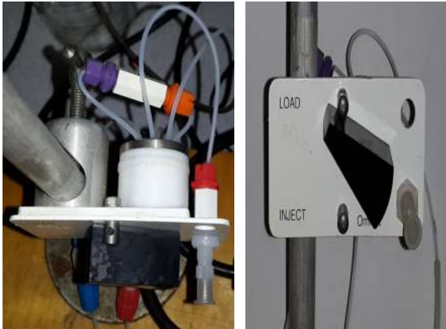
Figure 3-5: A picture of the top and side of the loop injector used in the HPLC set-up for the separation on the monolith
