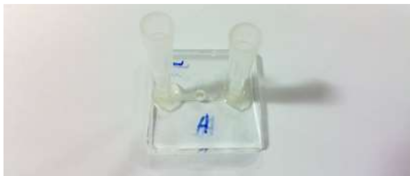
Figure 5-3: Eppendorf tips placed on the glass chip to hold solutions in place
