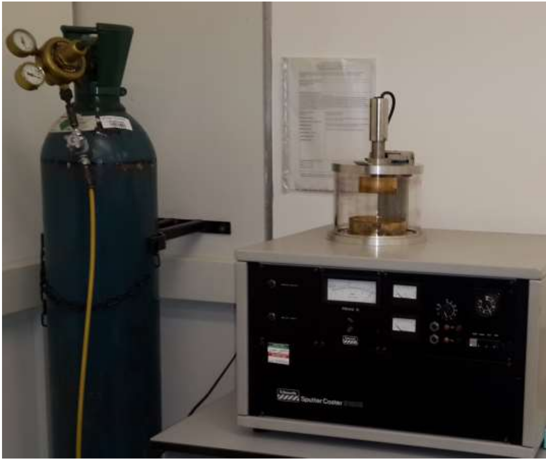
Figure 3-23: Edwards S150B gold-sputter coating instrument
