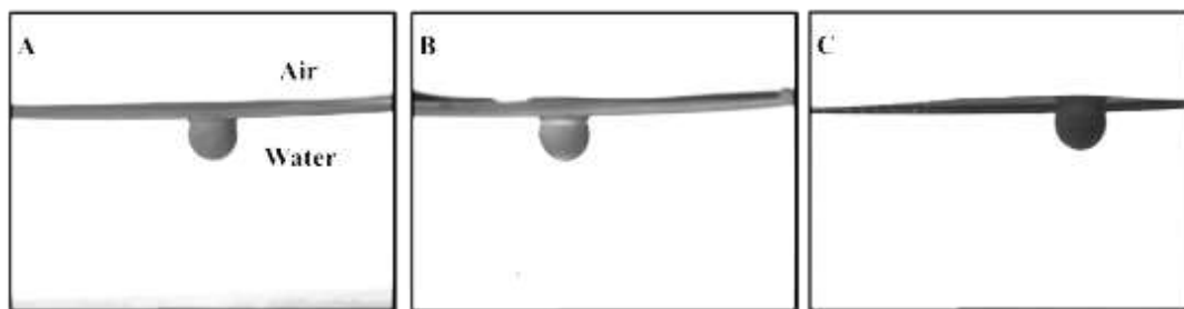
Figure 7.25. Side camera images from DSA 10 for water-wet supra-particles attached at the a/w interfaces for different sonication times in the ultrasonic bath after: (A) 3 min, (B) 6 min and (C) 9 min. The particles were initially attached at the a/w surface using a spatula.
