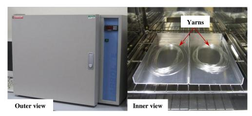
Figure 3-14 Fan-assisted oven used for fibre annealing. Inner view shows the yarns were placed in aluminium trays to ensure uniform heat treatment and prevent movement from air flow.
