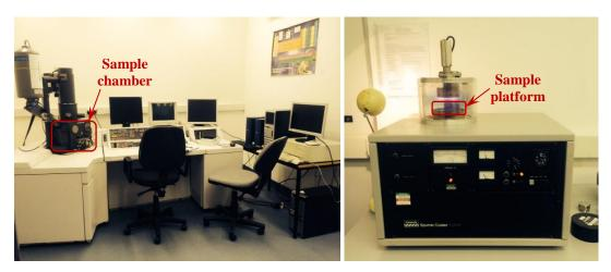
Figure 3-17 Equipment used for scanning electron microscopy: (a) SEM operation system; (b) sputter gold coater.
