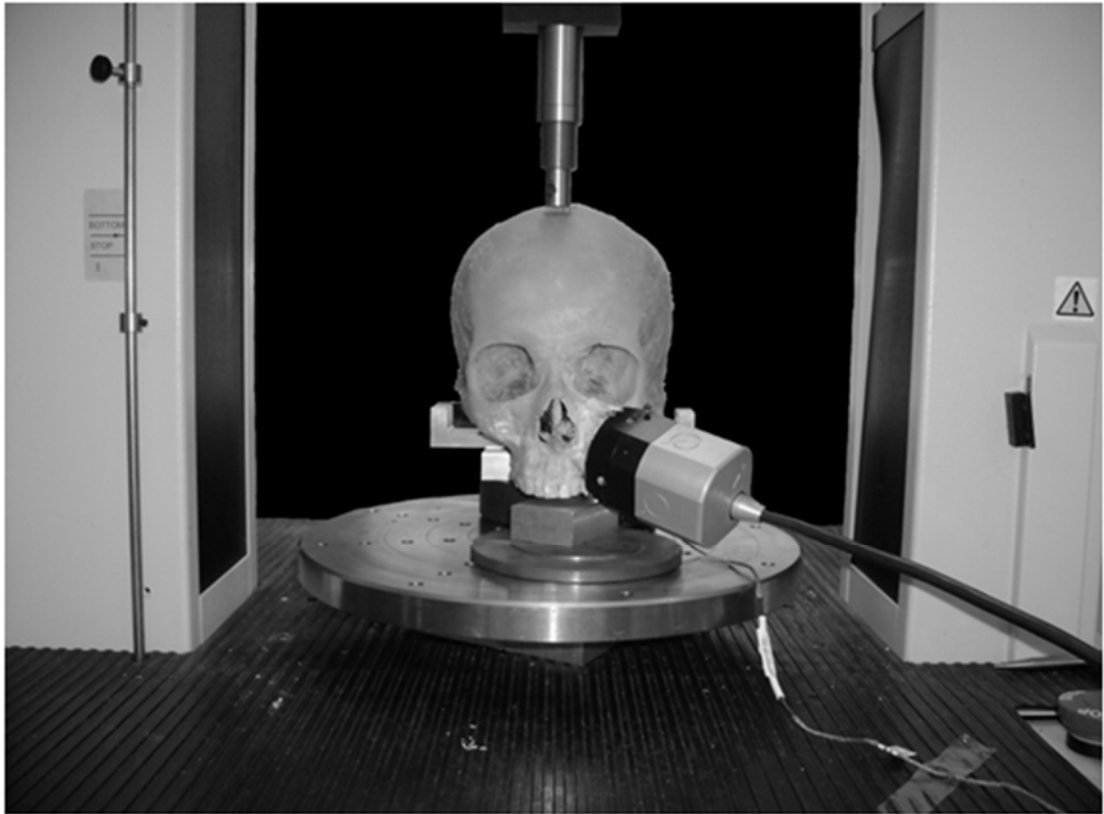
Figure 2-1: Experimental set-up of the skull used in the validation study.
