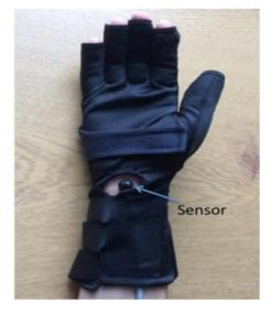
Figure 39: Positioning of the sensor at the wrist
