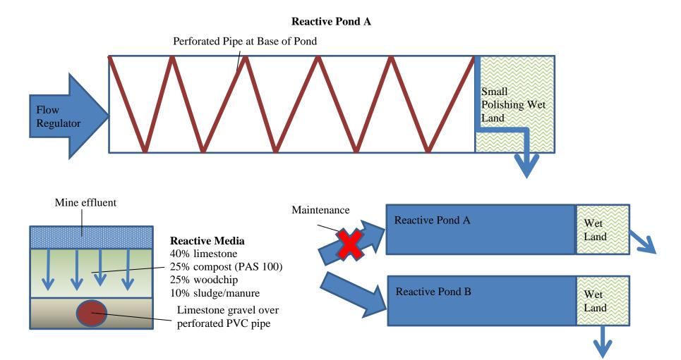
The configuration of the semi-passive bioreactors for the case study based upon the Hebden Beck site is shown Figure 6.6 and the individual components of the system are shown in Table 6.5.
