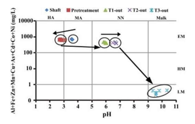
Figure 6.2:Modified Ficklin diagram for the different steps in the NFOL+DAS treatment. HA: high acidity, MA: moderate acidity, NN: near neutral, Malk: moderate alkalinity, EM extreme metallic, HN: high metallic, LC: low metallic T1: tank 1, T2: tank 2, T3: tank 3
