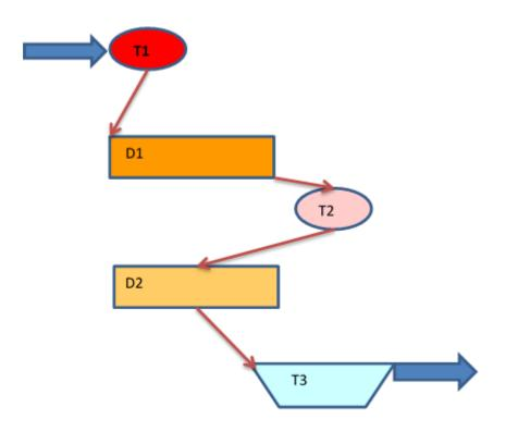
Figure 6.4: Passive HFO, based on DAS passive treatments system based upon (Macias et al., 2012b) T1: 3 m<sup>3</sup> Cylindrical fibreglass tank (3000 litres), T3: 0.168 m<sup>3</sup> rectangular fibreglass tank (168 L) (basal area 0.35 m<sup>2</sup>), D1-2: 6 m<sup>3</sup> decanting ponds, dug into the ground and isolated with UV proof plastic
