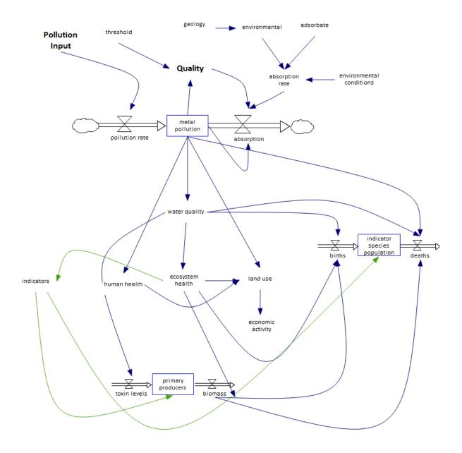
Figure 5.8: Simplifying simulation diagram for the impact point source of pollution at Hebden Beck (absorption refers to the rate of removal of metals by the selected remediation technology)
