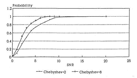
Fig(7.7b) Probability of crossing for Chebyshev filter.
