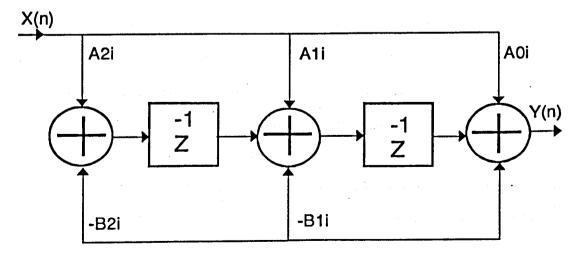
Fig[7.2] Structure of a biquad elements for use in implementing IIR filter.
