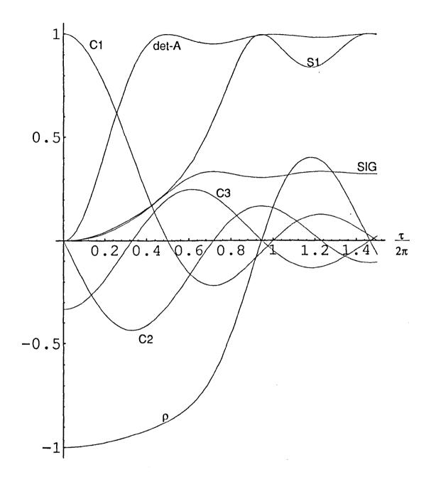
Fig[5.2] Normalised coefficient for Brickwall filter. C1=rx, C2= $\dot{r}$ Bx, C3= $\dot{r}$ Bx, S1=(1- $\rho^2$ ), SIG= $\sigma$ By, det-A=detA
