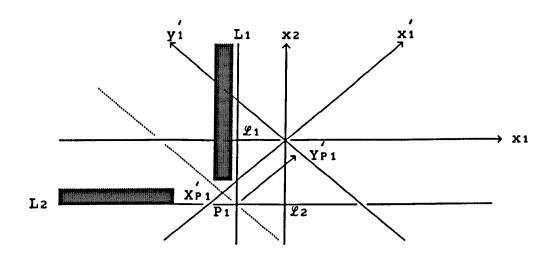
Fig[4.2] Condition for a positive slope (up-crossing) of level zero in time interval  $\Delta t_1$ .
