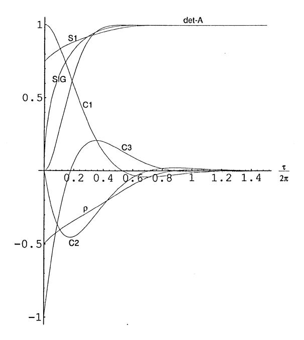
Fig[5.1] Normalised coefficient for Butterworth filter. C1=rx, C2= $\dot{r}_{Bx}$ , C3= $\dot{r}_{Bx}$ , S1=(1- $\rho^2$ ), SIG= $\sigma_{By}$ , det-A=detA
