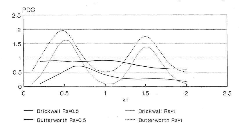
Fig[5.6b] PDC for SNR=1, for both filters with same time scaling.
