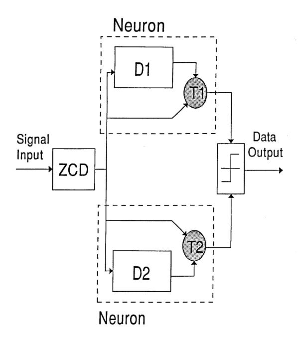
Fig[1.2] Binary FSK neural demodulator.
