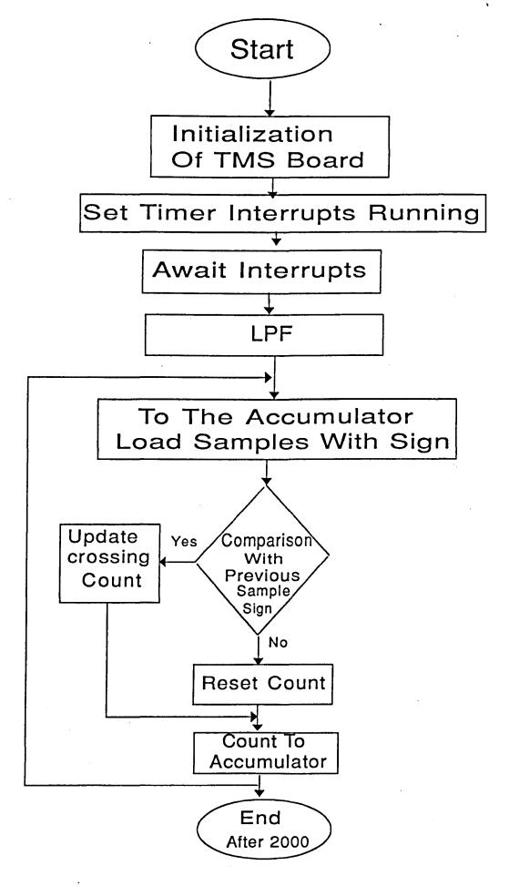
Fig[7.3] Zero Crossing detector flow diagram.
