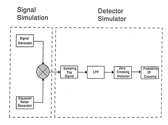
Fig[7.1] Block diagram of experimental set up.
