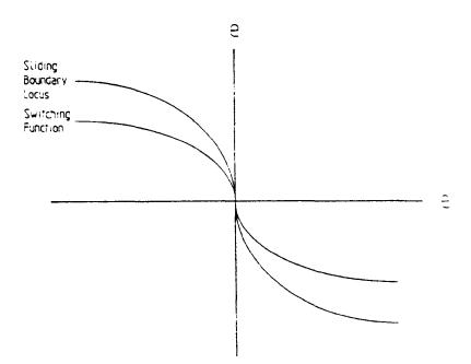
For a VSC system with input saturation it is impossible to obtain sliding behaviour outside the region of sliding for the equivalent relay system. If a controller is designed without consideration of this limiting effect, a switching surface may be selected which passes outside the sliding region, leading to non-sliding behaviour and possible overshoot.
