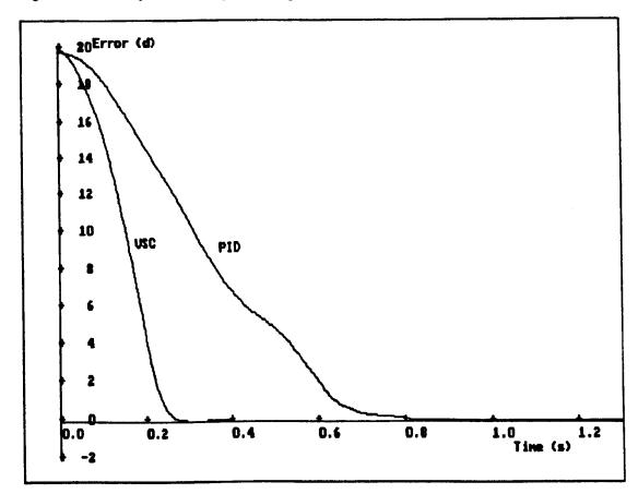
Figure 6.42 Comparison of speed using VSC and manufacturer's PID control
