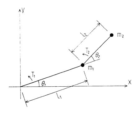
Applying Lagrange's equation, it is straight forward to derive the equation of motion for this system and it is shown in appendix 4 that the equation may be written:
