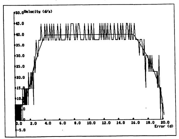
Figure 6.40 VSC with a piecewise linear switching function
