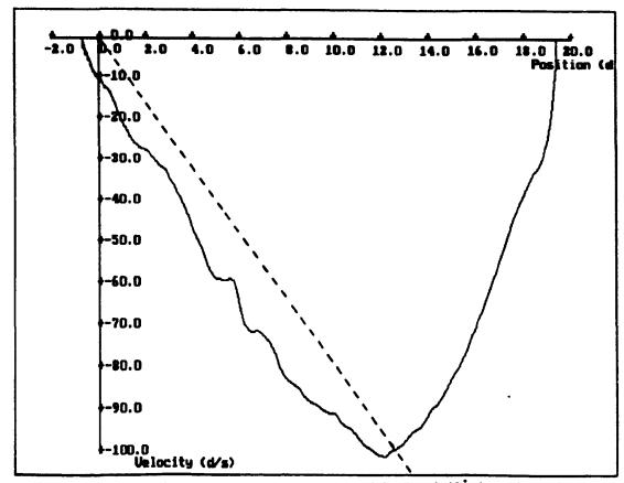
Figure 6.19 Response for controller with over-compensation of friction
