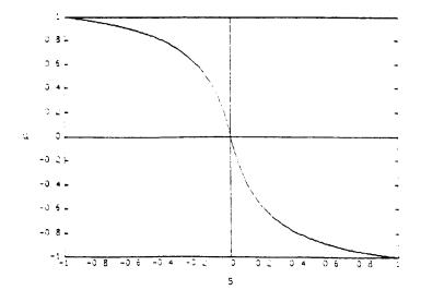
It should be noted that as the trajectory approaches the origin in this form of control the sliding sector becomes vanishingly small, returning us to the situation of discontinuous control. In order to rectify this problem a combination of sectors and bands may be adopted in the form shown in figure 2.15
