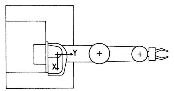
Both point-to-point and continuous path accuracy measurements were performed with the arm at a distance of 327mm from the highest point of it's travel.
