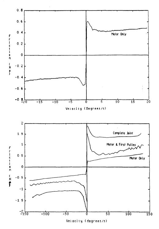
Figure 4.15 Frictional torque in the elbow joint of the RTX
