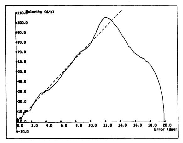
Figure 6.22 VSC with boundary layer and integral action  $(k_i = 37.2V/^{\circ})$
