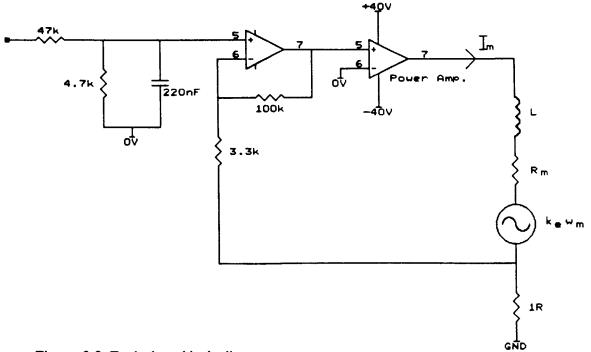
Figure 3.8 Circuit of current drive system with input filter
