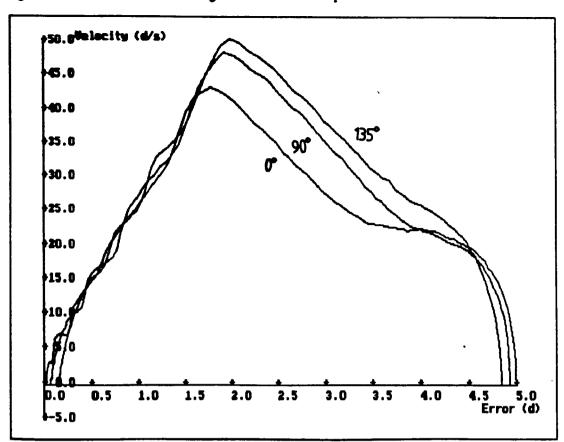
Figure 6.11 Effect of elbow angle on shoulder response
