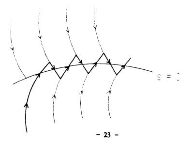
The precise form of the chatter is dependant on the nature of the unmodelled dynamics and the time delays present. Chatter is undesirable because it involves a large amount of control activity and may excite unmodelled dynamics. In addition, in mechanical systems, this high frequency oscillation may cause excessive gear wear and fatigue.
