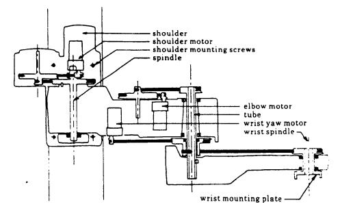
All the motors except that on the Z axis are of the same type, being DC permanent magnet brushed types with integral gearboxes. The reduction ratio in
