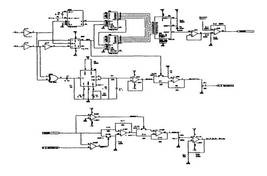
The control parameters are c, the switching line gradient, and  $\Psi$ , the controller gain; these are defined by VR<sub>1</sub> and VR<sub>2</sub> which were implemented using resistance boxes, to allow rapid variation.
