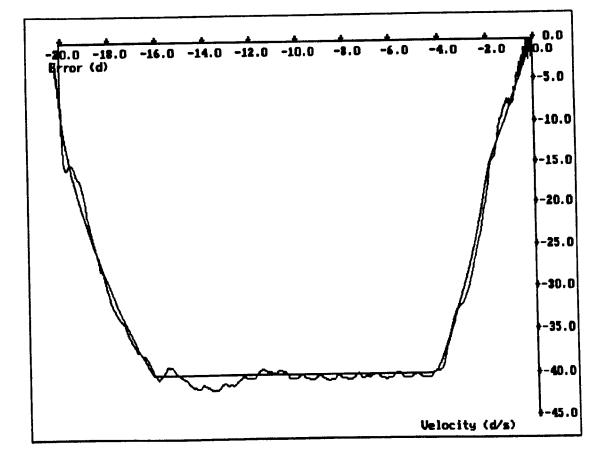
By combining all the compenents, it is possible to obtain good switching line following and improved robustness to parameter changes, as shown in appendix 7.1
