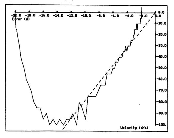
The deviation of the trajectory from the switching line has been significantly reduced by the removal of the discontinuous control signal, without an increase in the steady state error. Once again, the use of a large controller gain results in undesirable behaviour, as seen in appendix 7.2.
