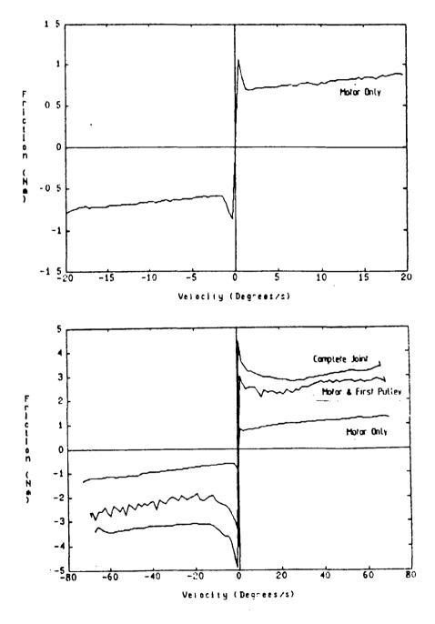
The frictional behaviour of the elbow joint is of a similar form to that found for the shoulder axis, as is seen from figure 4.15. An added consideration in the case of the elbow axis is that, since the drive to the yaw joint passes through this axis, an additional element of friction is caused by this drive. The extent to which this occurs is seen in figure 4.16 where the friction found in the complete elbow axis is plotted against speed, with and without the yaw axis drive connected.
