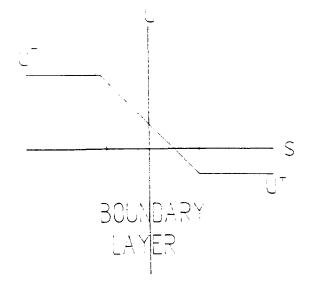
There are a number of variations on this idea such as using sliding sectors, as proposed by Zinober [Zinober,88] and Yeung [Yeung,88], where the phase plane is divided up as shown in figure 2.13, with switched control activity outside the sectors and a smoothed signal within.
