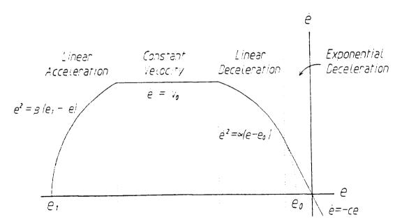
This type of switching function does provide a complete trajectory which is insensitive to parameter variations and disturbances. In order to assure sliding behaviour on all parts of the curve in the presence of these effect however, the curves must be sub time optimal, the degree of sub optimality being dependent on the extent of the disturbing influences.
