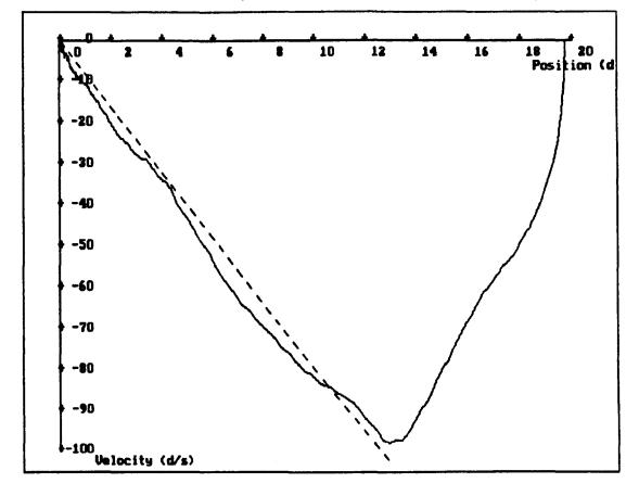
Figure 6.20 VSC with boundary layer and friction and acceleration compensation
