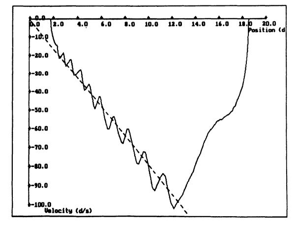
It is clear that chatter still remains with the friction compensated controller but the steady state error has been reduced to  $0.47^{\circ}$  in figure 6.14, compared with  $1.72^{\circ}$  for the system with no friction compensation, shown in figure 6.15.
