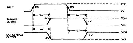
VOLTAGE WAVEFORMS ENABLE AND DISABLE TIME, THREE STATE OUTPUTS
