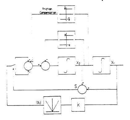
The friction is estimated as  $\hat{a}(x_2)$  which may include compensation for other effects, in addition to Coulomb friction. The maximum steady state error then becomes
