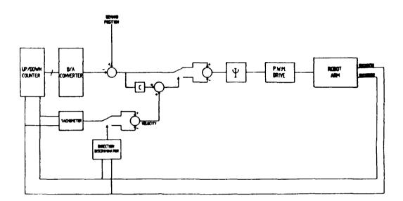
Figure 6.3 Circuit Diagram of the Hardware Implementation
