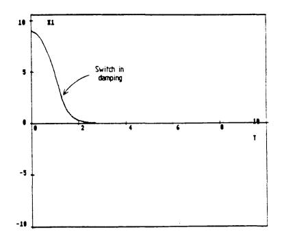
Figure 2.3 Trajectory of system with switched velocity feedback
