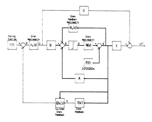
To facilitate the design of linear and nonlinear controllers blocks f(x) and Q(s) are included. The first of these allows any linear combination of functions of a single states to be fed back to the system input or, for switching controllers, into the switching block, Q(s), which then provides switched state feedback.
