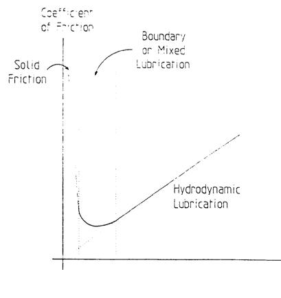
As the loading on the bearing increases the velocity at which fully hydrodynamic lubrication begins increases, due to the increased load on the lubricant film which tends to force lubricant out of the loaded region.
