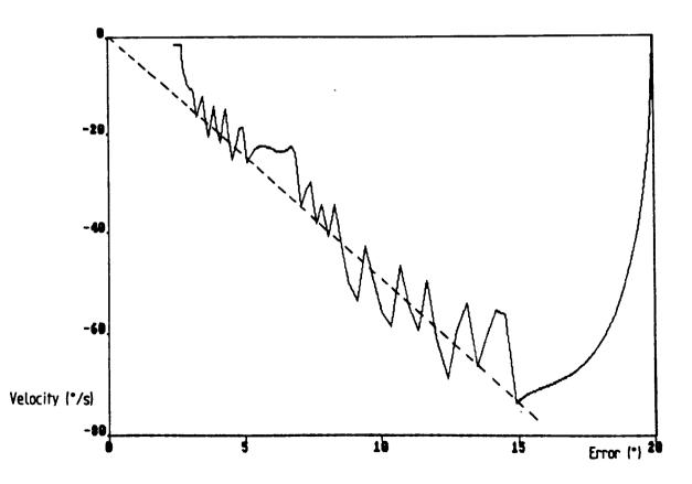
The reaching and sliding phases can be clearly distinguished, as can the chattering behaviour and the steady state error due to Coulomb friction. There is a significant steady state error, indicating the large amount of friction present in the drive system. This could be reduced by an increase in gain but only at the cost of increased chatter.
