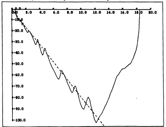
Figure 6.14 Response of Elbow joint with friction compensated controller
