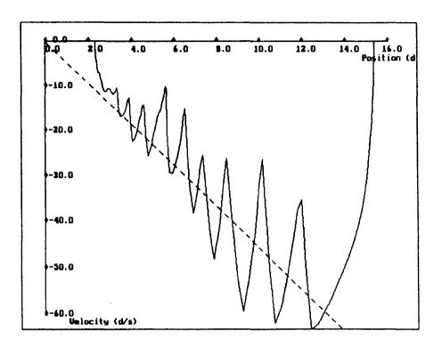
Figure 6.6 Effect of varying sampling rate in a simple VSC
