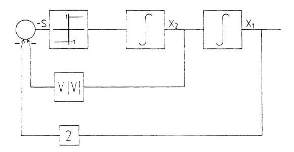
The nonlinear feedback defines a switching line in phase space given by the equation  $s = 2x_1 + x_2 |x_2| = 0$  and the system response depends on the position of the state point, relative to this line so that the dynamic equations are given by:
