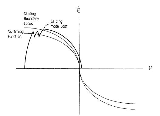
Figure 2.10 Loss of sliding due to chatter
