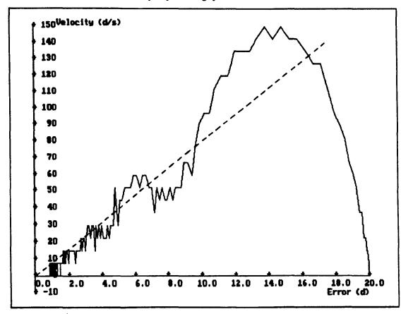
Figure 6.38 VSC with boundary layer using joint and motor mounted sensors
