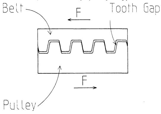
Figure 4.21 Meshing of toothed belt and pulley showing tooth gap
