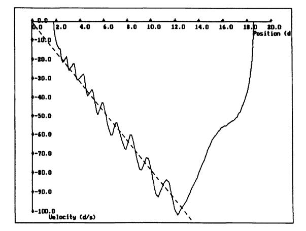
Figure 6.5 Response of a simple VSC implemented in software
