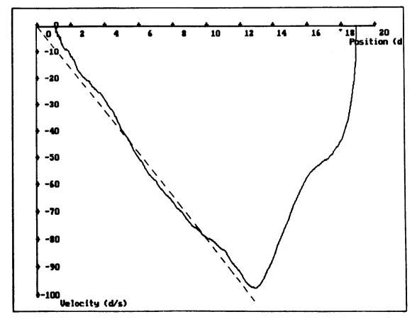
It will be seen that the trajectory remains close to the switching line for the majority of the trajectory, without chatter, but leaves the switching line as the origin is approached, leaving a steady state error of  $1.2^{\circ}$ . By introducing friction compensation at a level of 4.9V, equivalent to a torque of 2.54Nm, this response is modified to that shown in figure 6.18.
