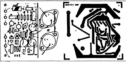
Figure 5 PCB component everlay and track layout
