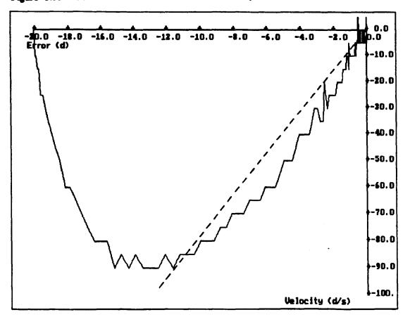
The final form of the controller, represented by the result shown in figure 6.35 gives close switching line following and a steady state error of  $0.05^{\circ}$ , corresponding to two encoder counts.
