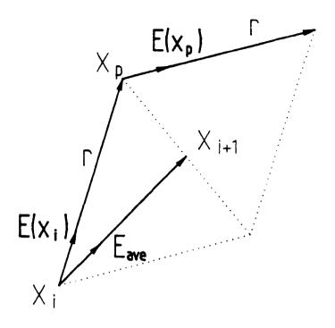
Thus the trajectory is extended a distance r in the mean direction of the derivatives at  $x_i$  and  $x_p$ .
