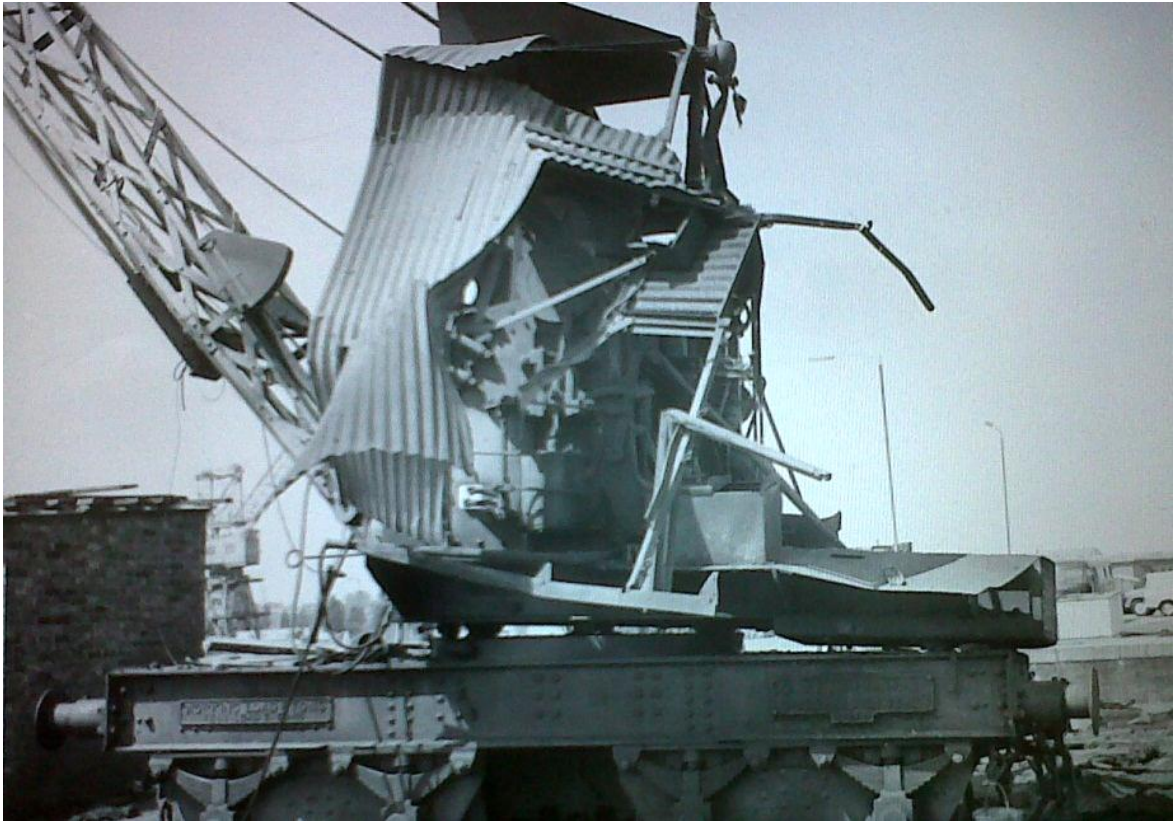
Figure 3.5a Travelling steam crane after the explosion of its vertical cross tube boiler on 4 July 1966. The corrugated iron that has been torn apart would have formed the cabin for the crane driver (see figure 3.5b below) and would also have housed the boiler. Source: RDL Accident Photograph Collection (black and white).
