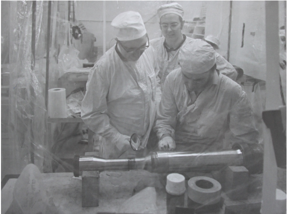
Figure 6.4: Workers in white overalls and cotton hats and gloves during nuclear refit. Note photograph taken through protective polythene. Presumably this was done to prevent any contamination being introduced to the working environment by the photographer.
