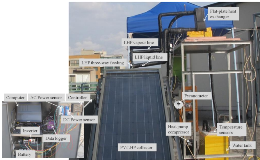
Fig. 6-1: On-site outdoor experimental rig
