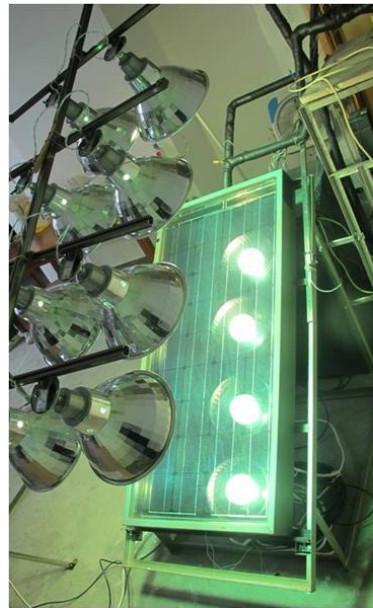
(a) PV/LHP module with single heat absorbing pipe
