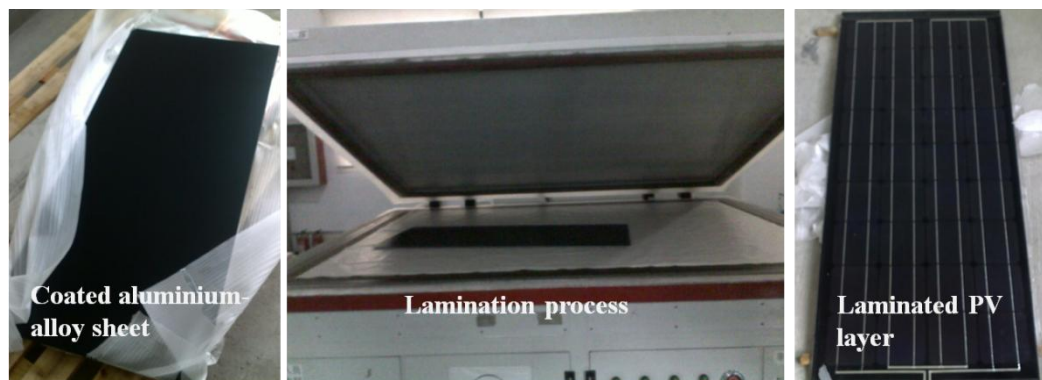
Fig. 5-1: Fabrication process of the Al-alloy-based PV layer
