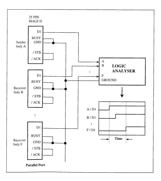
Figure 5.31 A Configuration for Transmission Time Check using a Logic Analyser
