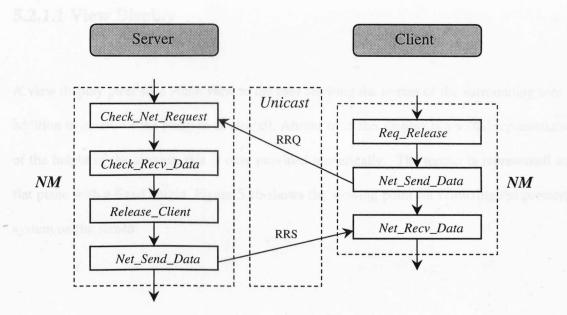
**Figure 5.15 Procedure of Release**
