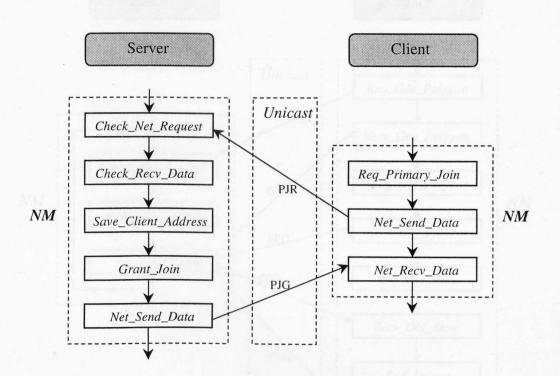
Figure 5.8 Procedure of the Initial Joi
