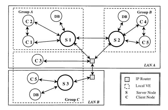
Figure 4.1 Networking Configuration of a DVM system
