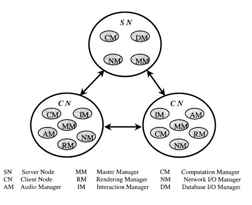
Figure 3.4 Components of DVM system
