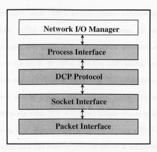
Figure 4.4 DVM Networking subsystem structure
