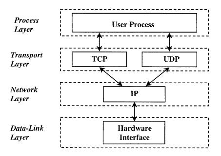
Figure 4.5 TCP/IP protocol suite using 4-layer model
