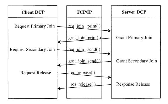
Figure 4.7 Message Exchange Sequence for Joining / Detach
