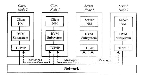
Figure 4.3 DVM Network Subsystem in the TCP/IP Protocol Suite
