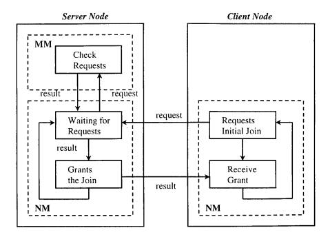
Figure 3.13 Routing Sequence for Initial Join
