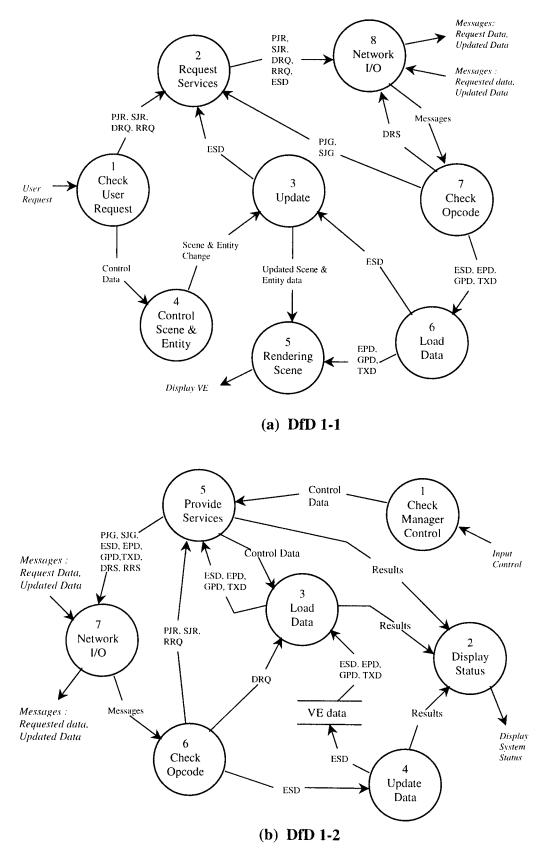
Figure 5.4 The level 2 DfD for the prototype system
