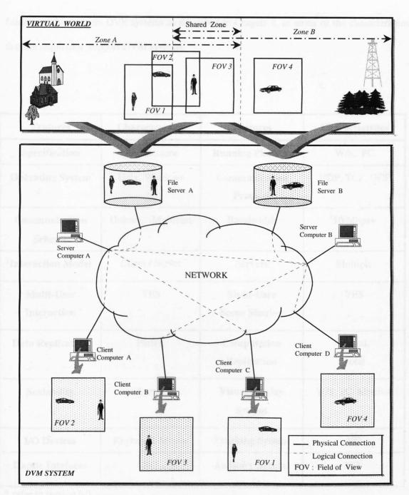
Figure 3.2 Basic Context Diagram of DVM system
