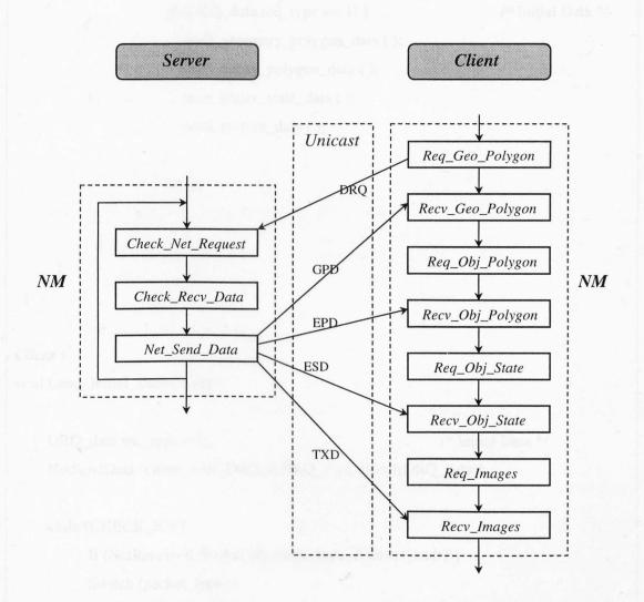
Figure 5.9 Procedure of the Initial Data Transmission
