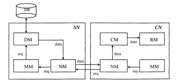
Figure 3.14 Routing Sequence for Transmission of Initial Data
