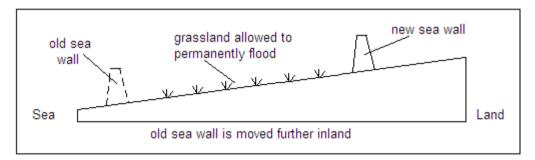
Figure 1.1 Process of managed realignment.
