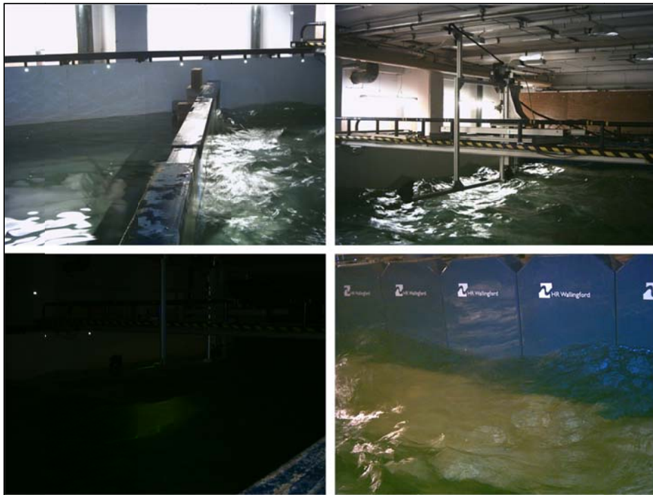
Figure 5.3 - Top Left: Boundary wall built to get the trapezoidal shape tank. Top Right: View across the tank of the gantry, the wire probes are mounted on either end of the aluminium frame and the laser guide can be seen at the top of the image. Bottom Left: The laser sheet during measurement. Bottom Right: Wave maker paddles.
