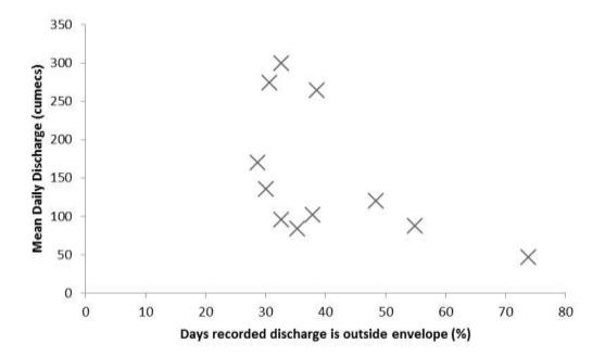
Figure 8.14 – Plot showing the mean daily discharge for each of the wet seasons between 1986 and 1996, and the percentage of days where the recorded discharge is either greater or lower than the modelled 95% confidence envelope of Pitman model modelled discharges, for the Bakoye catchment.
