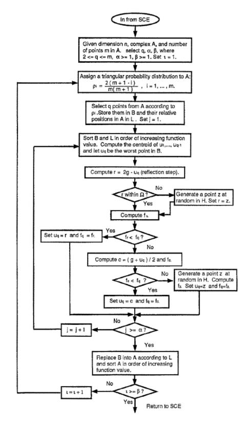
Figure 6.3 – Flow chart of the Competitive Complex Evolution (CCE) strategy, part of the SCE algorithm shown in Figure 6.2 (from Duan *et al.*, 1993).
