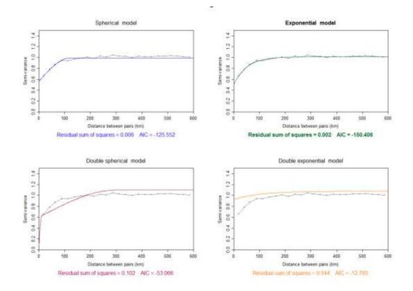
Figure 4.7 – The 'no-zero' rain field variogram fitted using different modelling methods.
