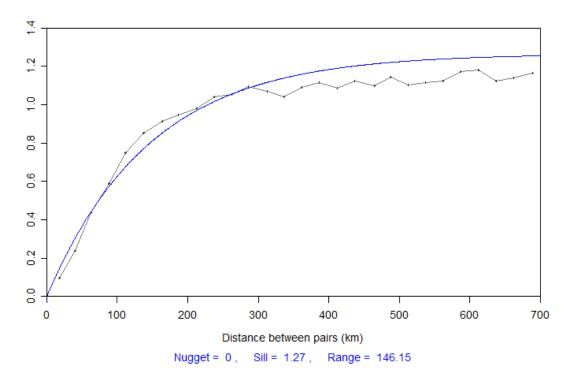
Figure 5.9 – Residual 'indicator' variogram and parameters for use in the TAMSIM algortithm.
