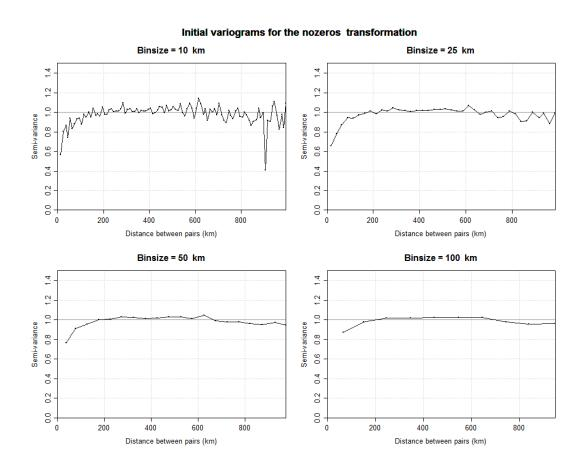
Figure 4.3 – Experimental 'no-zero' variograms generated by KrigeRain using different binsize settings.
