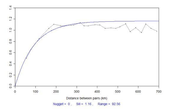
Figure 5.10 – Residual 'no-zero' variogram and parameters for use in the TAMSIM algorithm.
