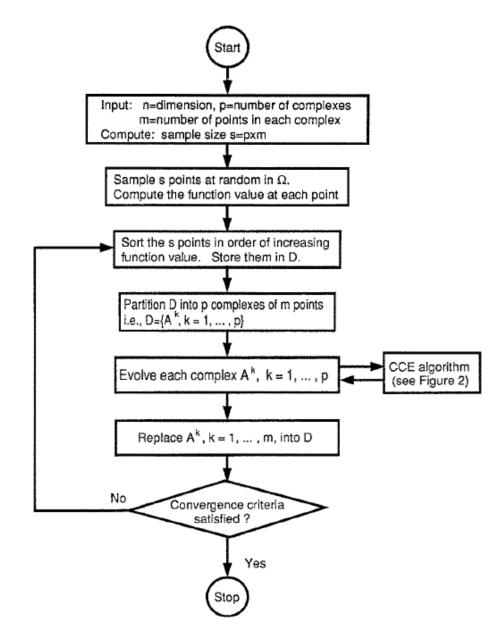
Figure 6.2 – Flow chart showing the main steps required for shuffled complex evolution (from Duan *et al.*, 1993) – The CCE algorithm can be seen in Figure 6.3.
