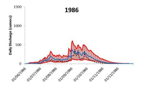
Figure 8.3 – Hydrograph showing the 95% confidence discharge envelope (in red) for 1986 for the Bakoye Catchment, driven by the TAMSIM ensemble SRFE using the EnsAll parameterisation. The solid blue line shows the deterministic TAMSAT1 discharge, and the dashed line shows the recorded discharge. (Note – 1986 represents the first year of the modelling and is therefore subject to the 'charging period')
