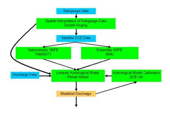
Figure 1.2 – Flow chart demonstrating the process used in this thesis, the main steps, and the methods employed. Blue boxes indicate the input data, green boxes the main steps and methods, whilst the brown box indicates the output.
