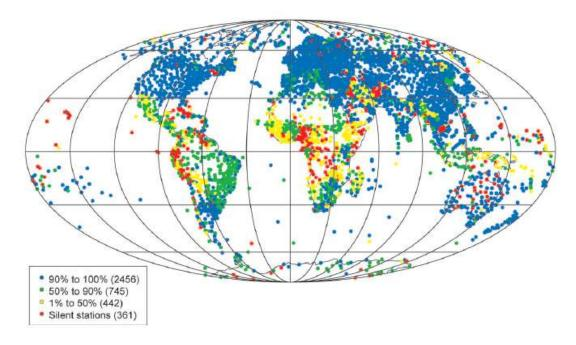
Figure 3.4 – The global distribution of raingauges that are part of the World Meteorological Organisation's (WMO) World Weather Watch (WWW) Regional Basic Synoptic Network (RSBN) in 2003. Each raingauge station is colour coded dependent upon its reporting rate (from Washington *et al.*, 2006).
