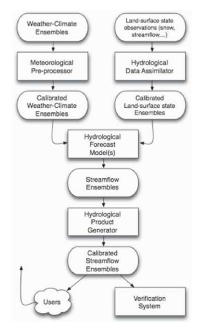
Figure 1.1 – A conceptual diagram of a possible end-to-end meteorological-hydrological ensemble streamflow system. The system allows for all sources of uncertainty to be accounted for (from Schaake *et al.*, 2007).
