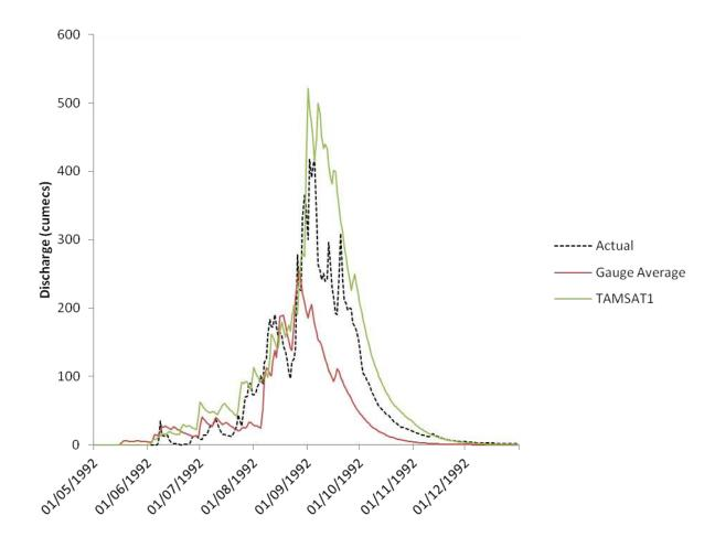
Figure 10.1 – Hydrograph showing the 1992 wet season for the Bakoye catchment. The recorded discharge is shown by the dashed line. The modelled output from the Pitman model calibrated and driven by the Gauge Average estimate for the period 1986-1996 is shown by the solid red line. The modelled output from the Pitman model calibrated and driven by the solid red line.
