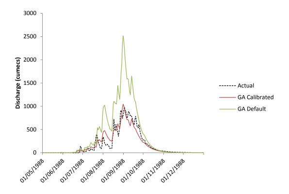
Figure 6.4 – Hydrograph showing the actual and modelled discharge from the Pitman model for the Bakoye catchment, for 1988. The dashed line shows the recorded discharge, the solid red line is the modelled discharge, driven and calibrated by the Gauge Average estimate of rainfall for the period 1986-1996, and the solid green line is the modelled discharge, driven by the Gauge Average estimate and using the default parameters.
