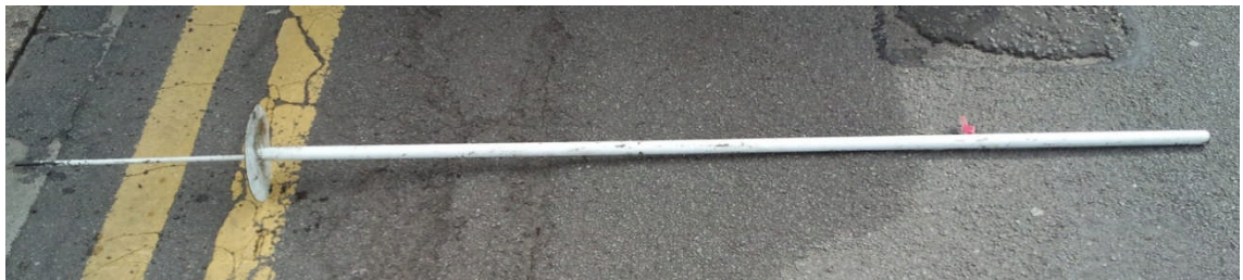
Figure 3.2 Content depth measurer, showing the thin plate which lies on top of the waste, the tip of the retractable inner rod and the red arrow indicating the depth.
