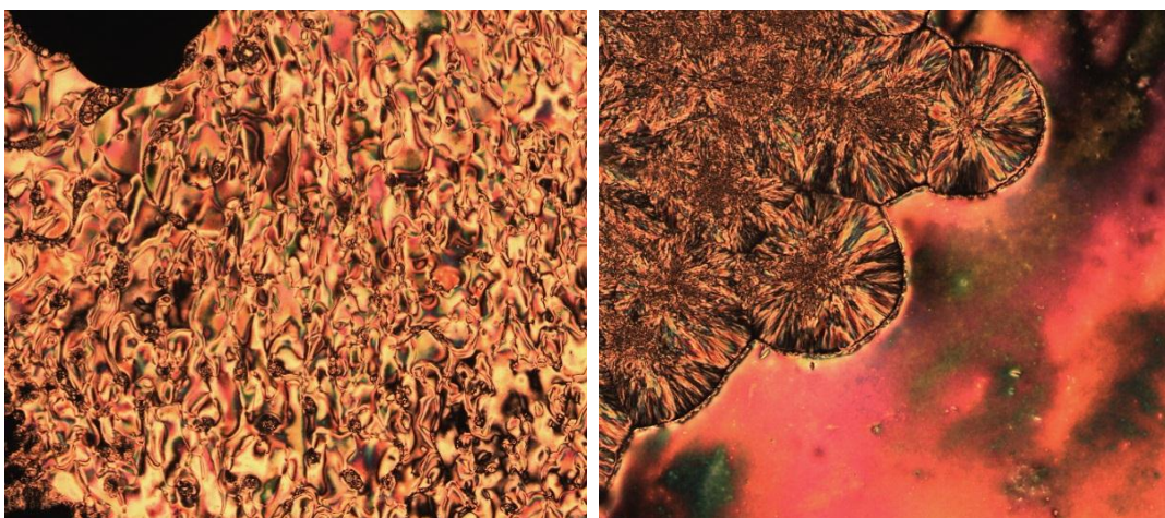
Figure 3.10 Polarised optical microscope images of 19c cooling from 30 °C.
