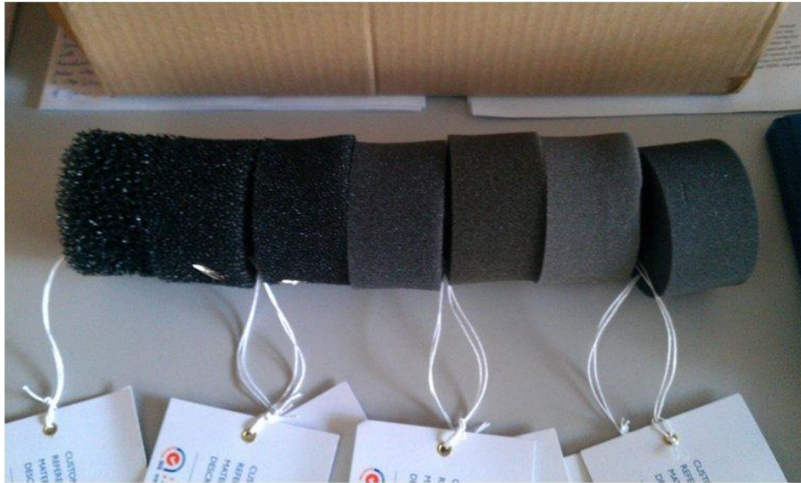
Figure 4.1: The seven different foam samples with a range of pore sizes from left to right of 10, 20, 30, 45, 60, 75 and 90 PPI
