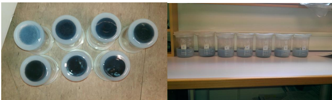
Figure 4.2: Phantoms suspended in agarose having undergone compression during preparation
