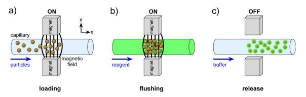
Figure 30 Trap and release method of magnetic particle handling in microchannels. a) Magnetic particles are loaded into the channel and trapped in a magnetic field, b) a sample or reagent is flushed over the trapped particles, allowing reactions to occur on the particles surface, before being washed with buffer solution, c) the field is removed and the particles released for downstream detection or further processing. Adapted from [99].
