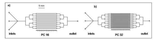
Figure 38 Schematic view of chips design for investigation on magnetic plug left device featuring a) PC16 and b) PC32.
