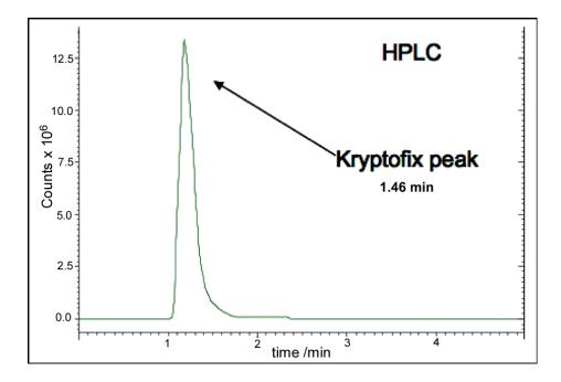
Figure 111 HPLC spectrum showing a typical chromatogram of Kryptofix.
