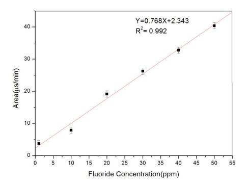
Figure 68 Calibration graph of area µs min<sup>-1</sup> vs series of concentrations of fluoride in the range 1-50 ppm.
