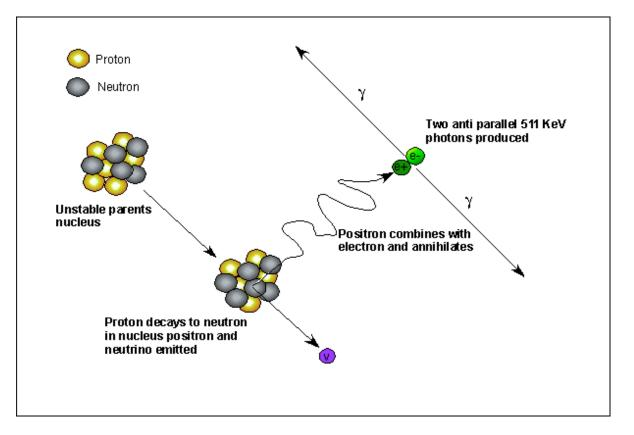
Figure 2 Schematic representation of positron emission and formation of 2 photons (gamma rays).
