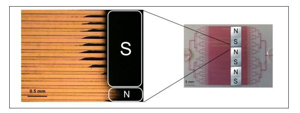
Figure 91 image of the plug formation on chip showing some of inner channels where no plug was formed possibly due to the weaker magnetic field gradient suggested using the FEMM simulation.
