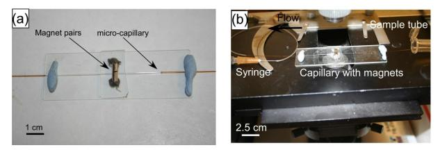
Figure 51 (a) Set-up of the glass capillary and the magnet pairs positioned on a glass slide, (b) Setup of the microfluidic device under the microscope.
