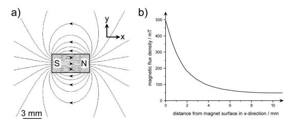
Figure 25 Characteristics of a typical rectangular magnet, illustrating a) the magnetic flux density, B, in and around the magnet, and b) the decrease in B with increasing distance from the magnet surface in the x-direction. Adapted from [99].
