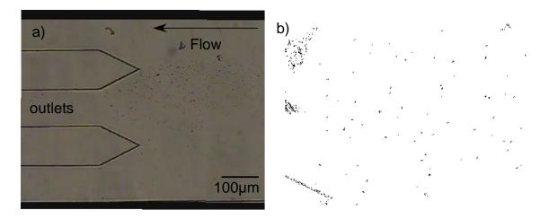
Figure 103 image of the video at the outlet of the chamber after 2 minutes showing particles stuck at the surface as proved by the background image, then the number of particles was counted before and after and percentage of sticking recorded.
