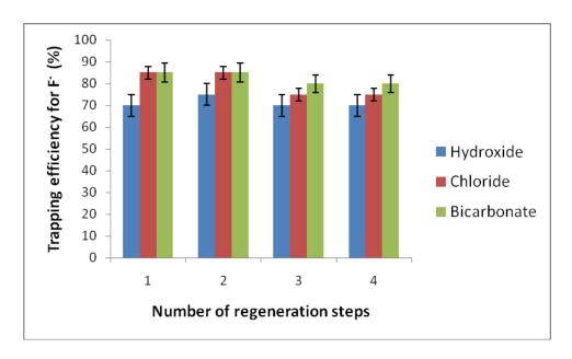
Figure 73 Graph comparing three different resin forms (hydroxide, chloride and bicarbonate) and their efficiency over a series of four runs.
