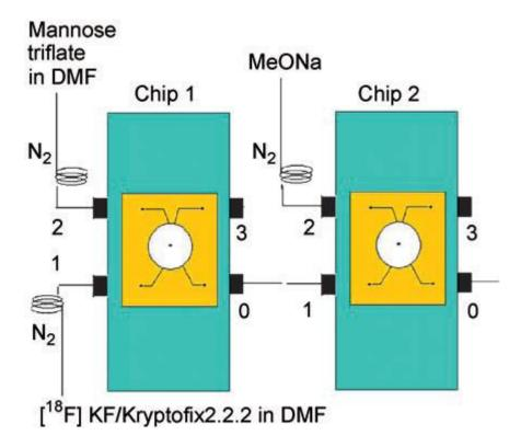
Figure 20 Schematic of the two microfluidic devices used by Gillies *et al.* Chip 1 radiolabelling of the mannose triflate, chip 2 base deprotonation [62].
