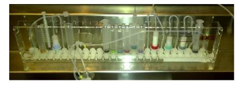
Figure 6 Image of a disposable cassette system with reagents and chemicals already loaded the image shows a cassette system for the GE "FastLab" [28].
