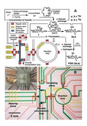
Figure 21 (a) Schematic representation of the microfluidic reactor circuit used for FDG production b) view of the device and optical micrograph from Lee *et al.*[64].
