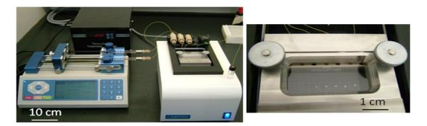
Figure 75 (left) Labtrix ® start system from Chemtrix BV. Temperature range -15°C to 190 °C for experiments. Pressure set to 15 bar. Also shown the microreactor (supplied with the instrument) in a holder that can be placed over the heated element. The tubing goes directly into the holder where it connected to the microreactor by `O` rings (made from Perlast®) so no leakage can occur. Courtesy of Victoria Hammond.
