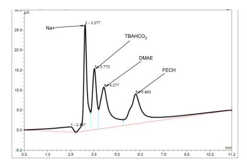
Figure 116 IC chromatogram of a mixture of DMAE and FECH and TBAHCO<sub>3</sub>separated with a CS18 cation column, 20 mM methanesulfonic acid 0.25 mL min<sup>-1</sup>.
