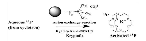
Figure 61 Principle of anion exchange process after the production of <sup>18</sup>F<sup>-</sup> from proton bombardment of <sup>18</sup>O water in a cyclotron. The fluoride ions are exchanged with the counter anions  $(CO_3^{2-})$  and subsequently eluted with high ionic strength salt  $(K_2CO_3)$  in the presence of acetonitrile and Kryptofix as phase transfer catalyst, to obtain the activated fluoride.
