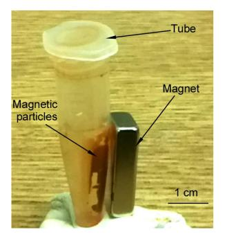
Figure 86 Photo of the off-chip set-up used to determine trapping and elution efficiency of fluoride, in this image is shown an Eppendorf tube with the box magnet placed on the side to allow the magnetic particles to be trapped on one side so that the supernatant can be analysed for presence of fluoride, Particles used in this image are Chemicell SiMAG-Q.
