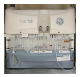
Figure 19 GE "FastLab" synthesiser by GE healthcare for synthesis of FDG [28].
