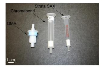
Figure 47 SPE cartridges commercially available. Silica based QMA from Water (50  $\mu$ m average particles diameter), Chromabond polystyrene cross linked with divinyl benzene (100  $\mu$ m average particles diameter) and silica based Strata SAX (60  $\mu$ m average particles diameter).
