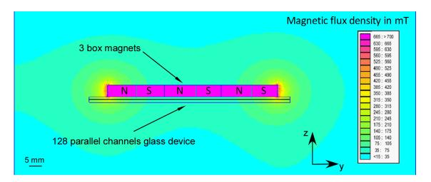
Figure 92 FEMM simulation of the magnetic flux density of 3 magnets facing opposite poles (10 x 10 x 5 mm<sup>3</sup> NdFeB magnets across the microfluidic chamber from a side-on cross-sectional view.
