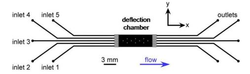
Figure 41 Schematic of chip design FL1, featuring an 8 mm x 3 mm reaction chamber, five inlets, and five outlets.
