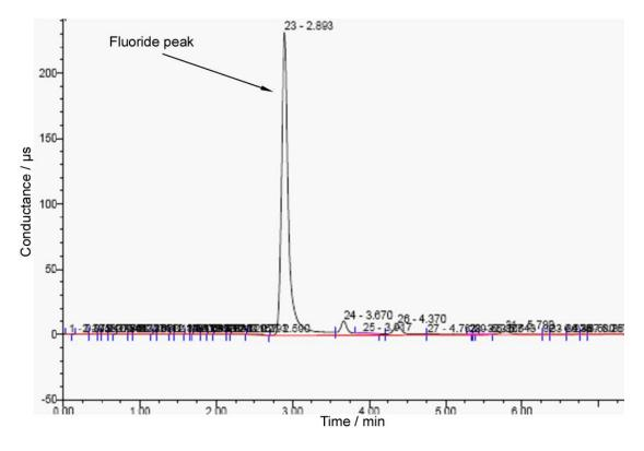
Figure 72 Chromatogram showing the effect of the carbonate ions on the resolution of the peaks. With 0.001 M  $K_2CO_3$  fluoride peak and other peaks present in water fully resolved without interference of carbonate.
