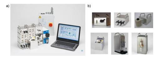
Figure 11 (a) Eckert & Ziegler modular system assembled and interfaced to a PC, (b) The individual components [36].
