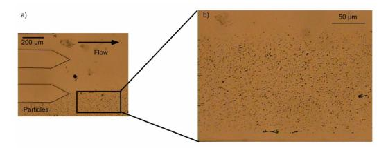
Figure 100 Image showing the Invitrogen SAX particles stuck in the glass device with no treatment.
