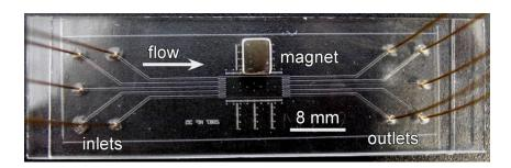
Figure 54 Chip design with the 4 x 4 x 5 mm<sup>3</sup> NdFeB magnet placed on top of the chip, next to the reaction chamber.
