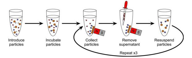
Figure 29 A typical reaction or separation using magnetic particles, where (1) the particles are introduced into the sample or reagent solution, (2) they bind to the target analyte/reagent, (3) the particles are collected using an external magnet, (4) the supernatant is removed and (5) the particles are resuspended in fresh buffer solution. Steps 3-5 are repeated several times to ensure any unbound material is removed from the particle surfaces. Adapted from [99]
