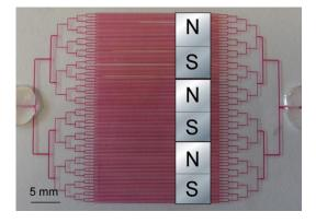
Figure 51 Image showing the device PC128 filled with red ink for visualization and the position and orientation of the NdFeB magnets.
