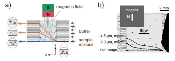
Figure 32 (a) Principle of on-chip free-flow magnetophoresis. A mixture of particles is introduced into a microfluidic chamber and deflected laterally by a magnetic field, allowing different particle types to exit the chip by different outlets [142]. (b) Experimental particle trajectories of 4.5  $\mu$ m and 2.0  $\mu$ m magnetic particles, as well as non-magnetic particles, demonstrating their separation as they traverse the chamber. Adapted from [113].
