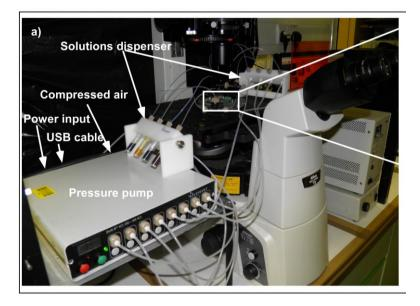
Figure 56 Full system set-up comprising of pressure pump connected to the chip and microscope for visualization.
