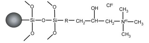
Figure 22 Example of a bound quaternary ammonium functional group with chloride as counter ion.
