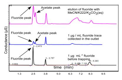
Figure 76 Chromatograms obtained for the trapping and elution of non-radioactive [<sup>19</sup>F]fluoride ions, showing 1µg mL<sup>-1</sup> fluoride before trapping (bottom), the diminished fluoride peak of waste solution collected during trapping (middle) and the full fluoride peak following elution (top).
