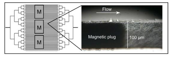
Figure 90 CAD image of the 128 parallel channels on the left and the formation of plug image downstream the magnet. Showing the position of the three magnets, which were always in the top middle of the glass device.
