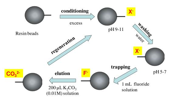
Figure 44 Schematic representation of fluoride activation; first conditioning of the resin, washing with water to neutralise the resin, trapping, elution and regeneration.
