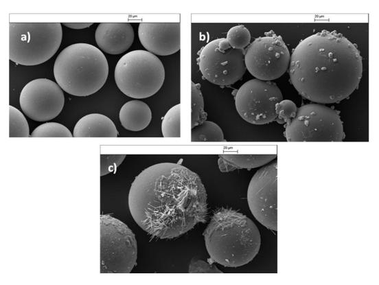
Figure 84 (a) SEM picture of PS-DVB particles. (b) SEM picture of PS-DVB particles after several treatment with [<sup>19</sup>F]fluoride. (c) SEM picture of PS-DVB particles after a series of treatment with 18 F fluoride, showing some crystal formation which was identified to be Na by elemental analysis due to non sufficient washing after the conditioning and regeneration steps.
