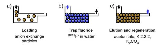
Figure 46 Pre-concentration of fluoride on trapped anion exchange particles, including (a) loading of the particles into a microfluidic device, (b) trapping of fluoride from solution and (c) elution of fluoride.
