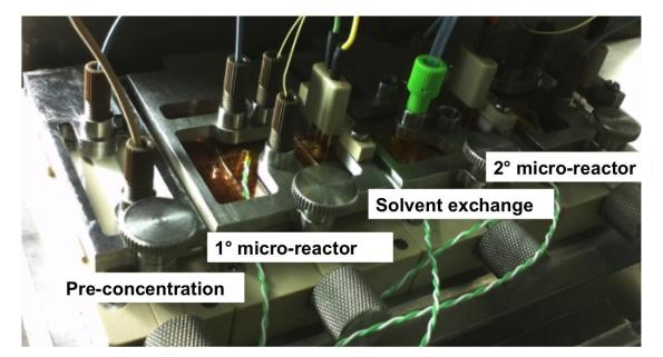
Figure 121 Image of the prototype modular system built by Siemens showing the four modules connected together in order the pre-concentration module, followed by the micro-reactor, the solvent exchange and the second micro-reactor.
