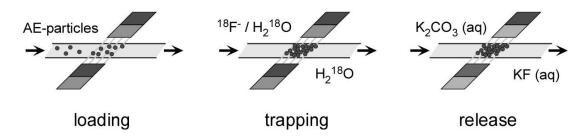
Figure 85 Schematic of the magnetic capture approach. Using an external magnet; fluoride can be trapped and subsequently eluted from the particle bed.
