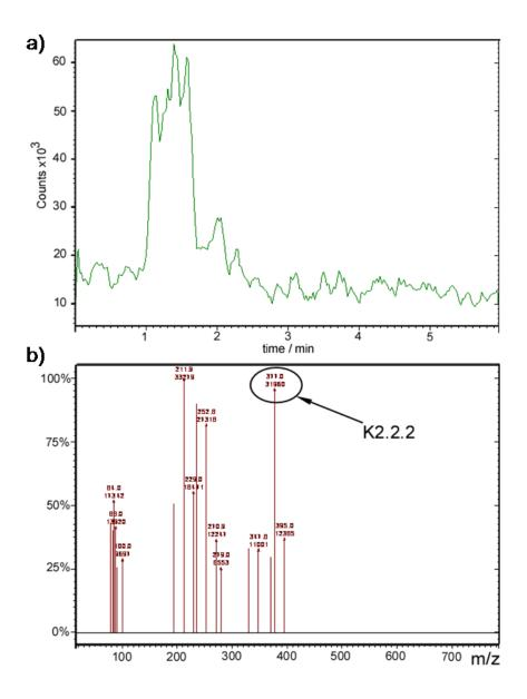
Figure 114. HPLC-MS spectrum of FDG showing very low count intensity for Kryptofix which was identified to be less than 100 ng.
