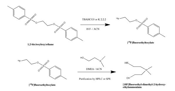
Figure 108 Synthesis of FECH in two steps reaction first fluoroethyltosylate is produced and then is reacted with excess of DMAE to yield the final FECH.
