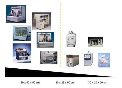
Figure 15 Comparison of the different radiochemistry modules described above in term of their size.
