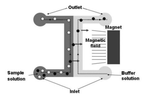
Figure 31 A common microfluidic method for continuous magnetic particle separation, known as a H-filter. A particle mixture is introduced into a wide channel alongside a buffer stream, and a
