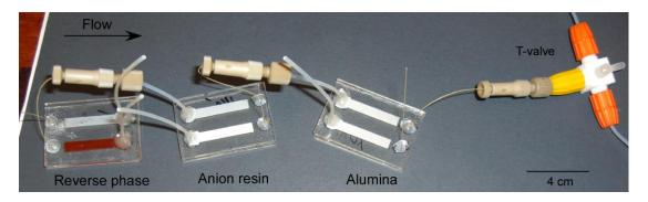
Figure 120 Image showing the three chips with different chromatography materials integrated and connected together used for FECH purification by trapping the byproduct and release the final product FECH.
