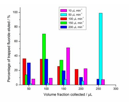
Figure 80 Elution of trapped fluoride from PS-HCO<sub>3</sub> particles at different flow rates. In all cases, 100 % of fluoride was eluted in the first 250  $\mu$ L collected from the chip, with higher flow rates typically affording faster elution times of the total fluoride.
