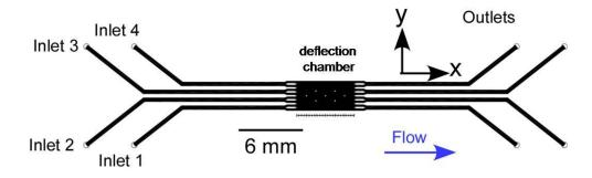
Figure 42 Schematic of chip design FL2, featuring a 6 mm x 4 mm reaction chamber, four inlets, and four outlets.
