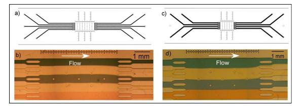
Figure 97 Laminar flow inside the chamber of two different chips design FDL1-FDL2, showing stable stream with minimal diffusion.
