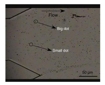
Figure 104 Image of a glass device inlet with APTES surface treatment where the different size of the dots represent the small one or two particles and the big dots a cluster of two or more particles agglomerate.
