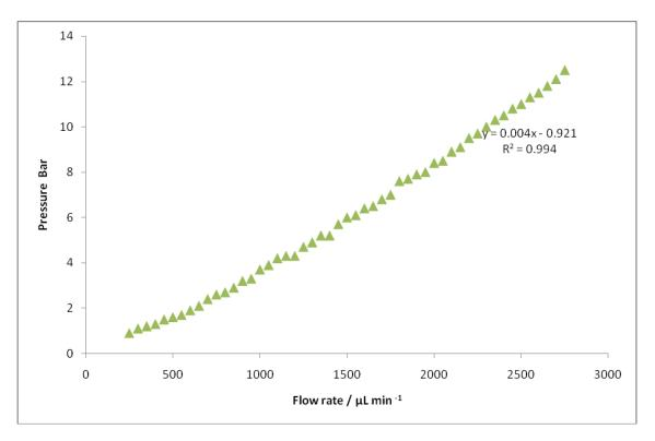
Figure 79 Calibration graph of the flow rate  $\mu$ L min<sup>-1</sup> vs pressure / bar.
