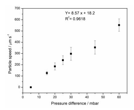
Figure 98 Plot of the particles speed  $\mu m s^{-1} vs$  pressur difference between inlets and outlet, particles used were Dynabeads M280.
