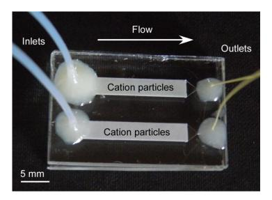
Figure 117 Image of glass device used for FECH removal showing the two chambers filled with approximately 20 mg each of cation exchange particles extracted from a CM cartridge from Waters UK
