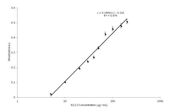
Figure 110 Calibration curve of the log scale of the concentration of standard Kryptofix solution (10  $\mu$ L) + acidified iodoplatinate reagent (10  $\mu$ L) and 800  $\mu$ L water vs the absorbance measured at  $\lambda$  365 nm.
