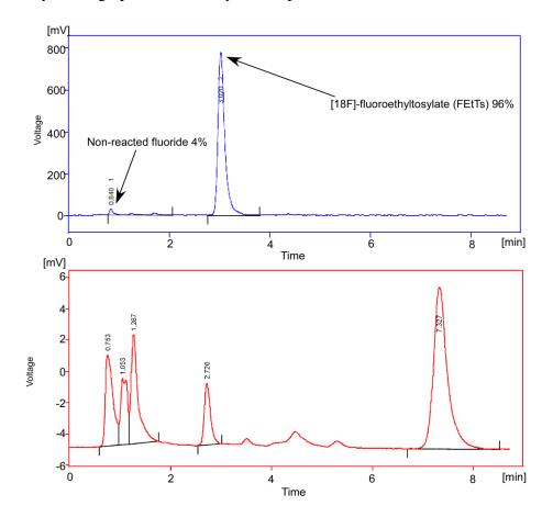
Figure 82 Typical Radio-HPLC profile for the labeling of ethyl ditosylate (EtDT) to yield [<sup>18</sup>F]fluoroethyltosylate. The top trace represents the radioactivity , and it shows the percentage of unreacted fluoride against the percentage of product formed, while the bottom trace represents the UV absorbance at 254 nm showing the unreacted EtDT peak ( $R_t = 7.3min$ ).
