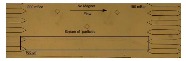
Figure 105 Image showing a stream of MyOne weak cation exchange particles flowing with very limited sticking from inlet to the outlet without magnet.
