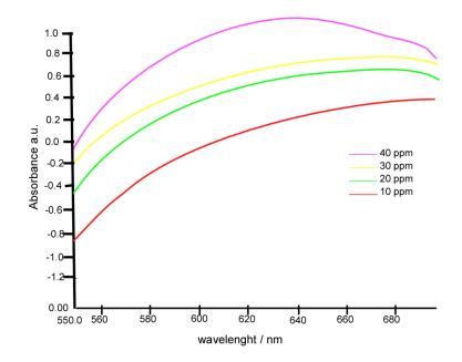
Figure 66 Absorption spectra of fluoride (10-40 ppm) and K<sub>2</sub>CO<sub>3</sub> (0.25 M) at 625 nm.
