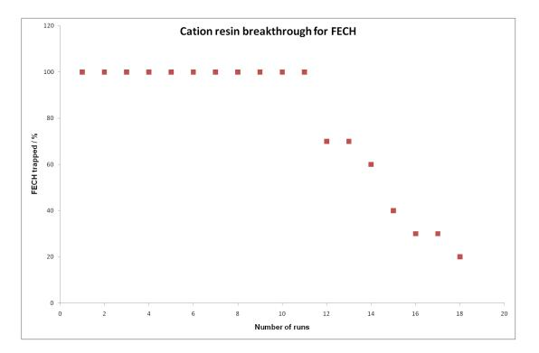
Figure 118 Graph showing the % of FECH trapped vs the number of runs which equal to 10  $\mu$ g mL<sup>-1</sup> per run.
