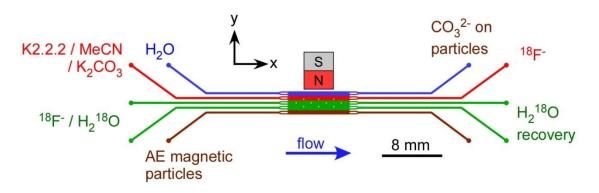
Figure 96 Continuous flow magnetic approach showing the principle of the multi laminar flow regime where AE particles are introduced into the reaction chamber and deflected *via* magnetic field (left). The green streams show the trapping while the red stream shows the elution of the fluoride.
