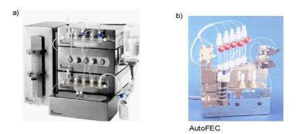
Figure 13 (a) The Scintomics modular system, (b) The "AutoFEC" modular systems for synthesis of FEC [39].
