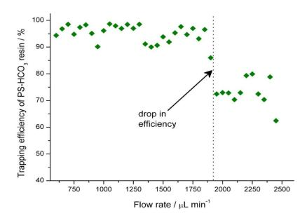
Figure 78 Graph showing the efficiency of the fluoride trapping onchip (%) vs flow rate  $\mu$ L min<sup>-1</sup> showing a decrease in efficiency of about 15-20 % after flow rate of 1800  $\mu$ L min<sup>-1</sup>.
