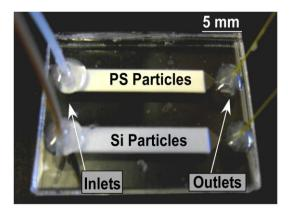
Figure 48 Dam structure device filled with two different anion exchange particles namely; silica (Si) and polystyrene (PS).
