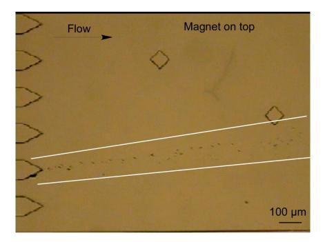
Figure 106 Image showing MyOne weak cation exchange particles deflected across the chamber towards the outlet in presence of a magnet.
