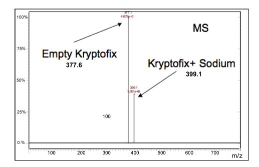
Figure 112 Typical MS spectrum of Kryptofix showing the empty kryptofic at 377 m/z and the sodiated Kryptofix at 399 m/z.
