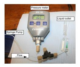
Figure 49 Set-up used to measure the pressure within the chamber of the packed bed device.
