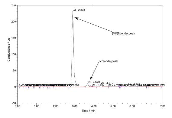
Figure 67 Chromatogram of a 30 ppm [<sup>19</sup>F]fluoride standard showing the retention time for [<sup>19</sup>F]fluoride at 2.893 minutes.
