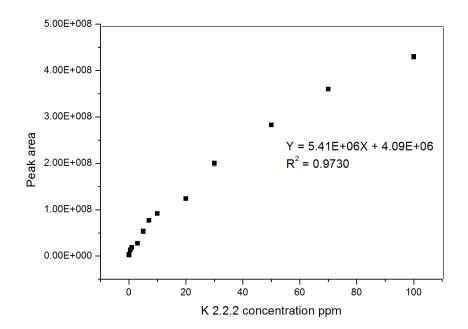
Figure 113 Concentration of kryptofix standards (0.1- 100 ppm) vs peak area measured with HPLC-MS.
