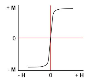
Figure 27 Magnetisation (M-H) curve for a superparamagnetic nanoparticle. As the applied field increases, so too does the particle magnetisation, until it is saturated. material, there is no magnetic remanence, meaning that upon removal of the field the particle essentially becomes non-magnetic.
