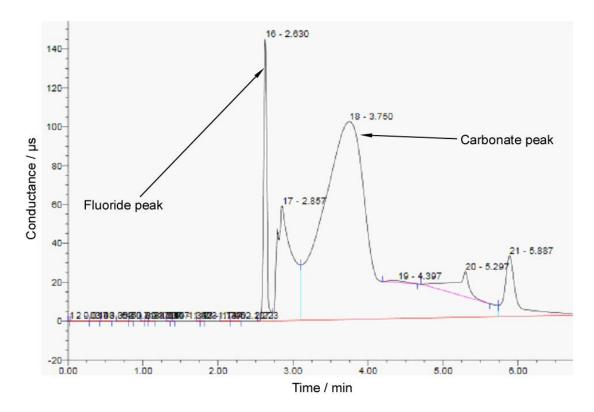
Figure 71 Chromatogram showing the effect of the carbonate ions on the resolution of the peaks. With  $0.01 \text{ M K}_2\text{CO}_3$  the fluoride peak is resolved, but the interference is still present for further detection of other ions.
