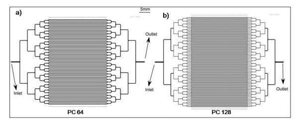
Figure 39 Schematic of chips design, featuring a) 64 parallel channels (PC64) and b) 128 channels (PC128).
