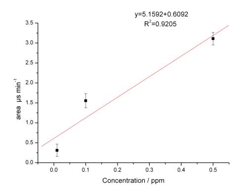
Figure 69 Determination of the LOD for [<sup>19</sup>F]fluoride using ion chromatography.
