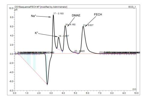
Figure 115 IC chromatogram of a mixture of DMAE and FECH separated with a CS18 cation column, 20 mM methanesulfonic acid 0.25 mL min<sup>-1</sup>.
