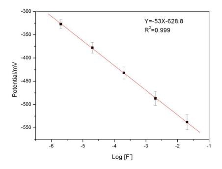
Figure 63 Calibration graph of Potential/mV versus the logarithm of [F<sup>-</sup>].
