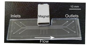
Figure 53 Glass chip featuring a box magnet 20 x 10 x 5 mm<sup>3</sup> within the glass cut out.
