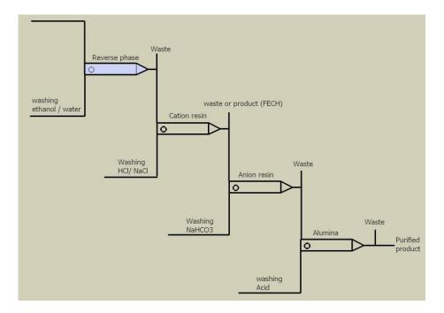
Figure 119 Schematic of four different micro-chambers independently connected where it will be possible to redirect the liquid solution in the desired chamber by using a valve or T junction to allow multiple radiotracers purification and subsequently the regeneration of each individual material.
