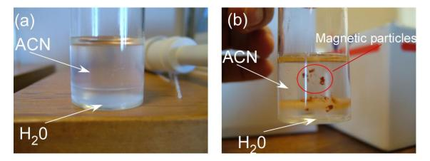
Figure 99 a) Separation of water-acetonitrile layers. b) Pulling of 3  $\mu$ m particles from water to acetonitrile with small permanent magnet.
