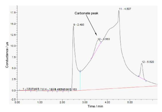
Figure 70 Chromatogram showing the effect of the carbonate ions on the resolution of the analytes at  $0.1 \text{ M K}_2\text{CO}_3$ .
