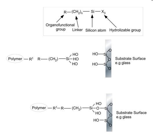
Figure 58 The deposition of silanising agents onto a glass substrate. The example shows an alkoxysilane featuring three hydrolysable methoxy groups.
