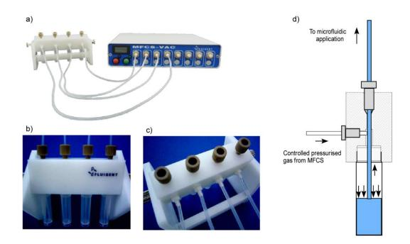
Figure 55 a) Schematic of the Fluigent pressure pump with the fluiwell + the reservoirs, b-c) image showing the front and back of the fluiwell (vials rack), d) showing the principle of the flow of the liquid via pressurized gas [165].
