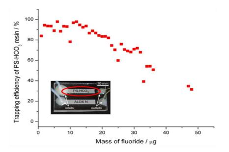
Figure 77 Breakthrough plot of the anion-exchange chip showing the trapping efficiency versus the amount of [<sup>19</sup>F]fluoride ions introduced into the chip. As the mass of fluoride was increased, the trapping efficiency decayed linearly as the number of trapping sites on the particles decreased. The maximum capacity of the anion exchange particles (Chromabond PS-HCO<sub>3</sub>) before loss of efficiency was determined to be 0.55  $\mu$ g mg<sup>-1</sup>.
