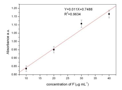
Figure 65 Calibration graph of absorbance vs concentration of fluoride.
