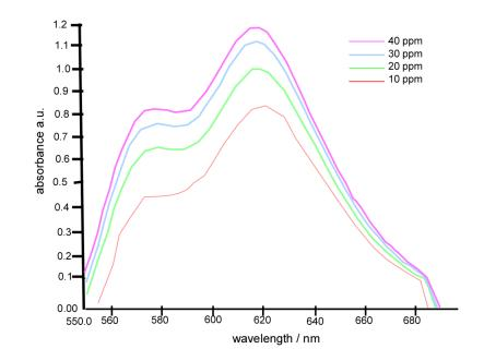
Figure 64 Absorption spectra at 625 nm of different fluoride concentrations (10-40 ppm).
