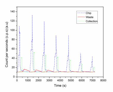
Figure 81 Seven consecutive runs of the trapping and elution of radioactive [<sup>18</sup>F]fluoride ions. Counts per second (c.p.s) was measured by three independent radioactivity detectors: on the chip (blue / dashed line), in the collection vessel after elution (green/ dotted line), and in the waste vessel (red / solid line).
