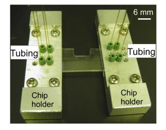
Figure 57 Chip holder featuring a glass device with cut out for magnet.
