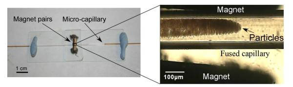
Figure 87 Single on capillary formation of plug at 120 µL h<sup>-1</sup>.
