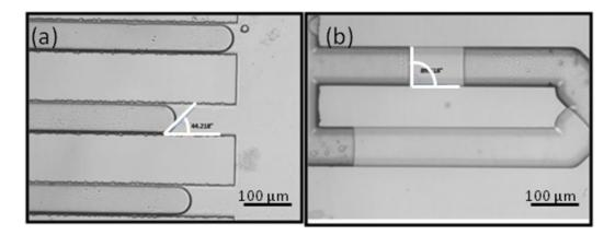
Figure 101 (a) Contact angle measurement using water/air interface without silanisation(°44.218), (b) after silanisation (°89.518).
