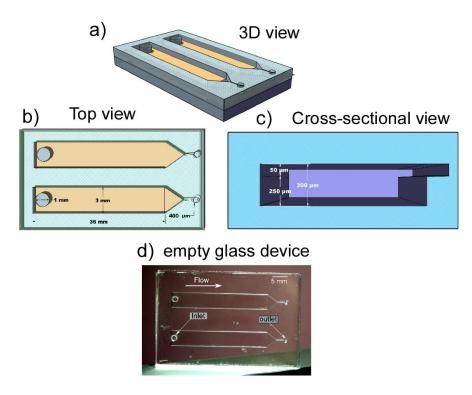
Figure 40 Schematic view of the dam structure chip device. a) 3D view, b) top view featuring dimension of the chamber and holes, c) cross sectional view featuring the depth of the double etched plates and d) a photo of the empty glass chip.
