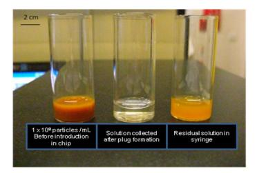
Figure 88 Magnetic particles suspensions (left) before introducing in chip as very dense concentrated solution, (middle) solution collected at the outlet of the 128 paralle channels showing the most of the particles have formed magnetic plugs, (right) residual particles at the end of the experiment found at the bottom of the syringe.
