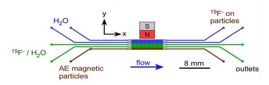
Figure 52 Schematic of the set-up of chip design for performing fluoride trapping in continuous flow. Magnetic particles were pumped into inlet 1, and fluoride ion in solution in inlet 2-3.
