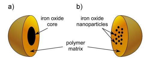
Figure 28 Cross-section of two types of superparamagnetic microparticle: a) an iron oxide core is encased in a polymer matrix, and b) iron oxide nanoparticles are dispersed throughout the polymer matrix, before being sealed inside with an extra layer of polymeric material.
