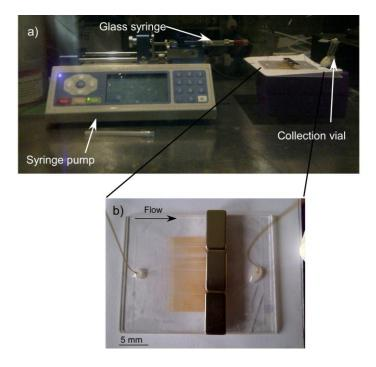
Figure 95(top) set-up of the on-chip trapping and elution of [<sup>18</sup>F]fluoride *via* plug formation of magnetic particles, showing a syringe pump, glass syringe and glass device, through a glass window for radioactivity shielding. (bottom) image of the glass device at the end of the experiment showing the brownish color given by the particles on the left and the clear side after the magnet on the right.
