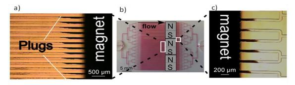
Figure 93 Photographs of magnetic particle plugs formed on chip (a) upstream from the magnet, (c) downstream from the magnets, (b) image of the 128 parallel channels device filled with red ink for visualization and showing the position and orientation of the NdFeB magnets.
