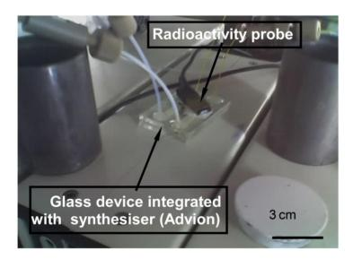
Figure 36 Image of the microchip device (packed bed microchip) integrated with the Advion Nanotek LF, showing the microchamber glass device and one of the three radiodetector probes placed on top the device for real time monitoring of the radioactivity.
