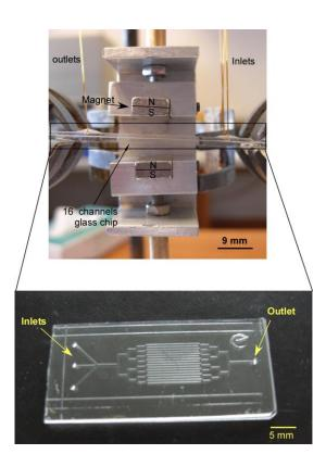
Figure 89 (top) Set-up of the magnet pairs to form plug, magnet held in place) by a clamp and placed on top and bottom of the glass device (at distance of 2 mm from the glass device for magnetic field improvement. (bottom) Image of the 16 parallel channels glass device.
