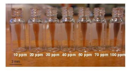
Figure 60 Image of the setup for of the colour change reaction between K2.2.2 and iodoplatinate reagent.
