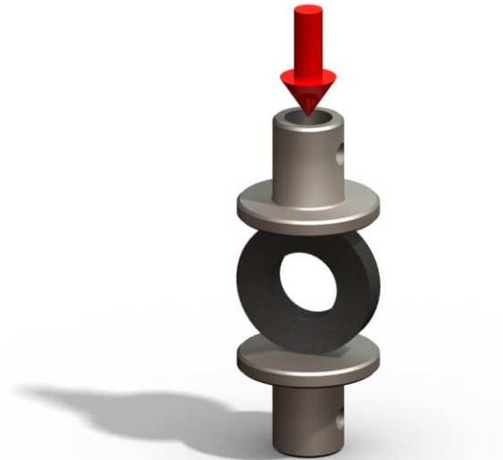
Figure 3.5: Schematic illustration of a brittle ring loading scenario.
