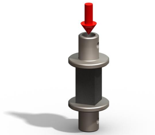
Figure 3.2: Schematic illustration of simple compressive loading scenario.
