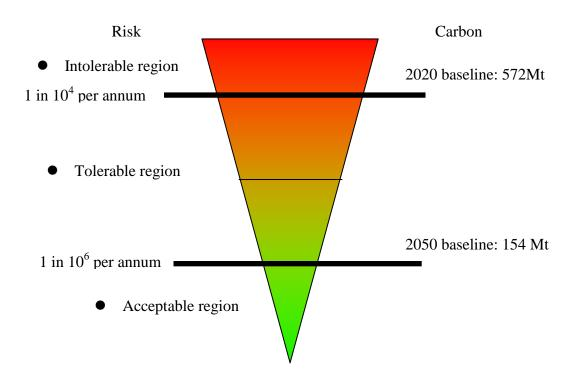
Fig.6.2. Intolerable, tolerable and acceptable regions of risk and carbon footprint
