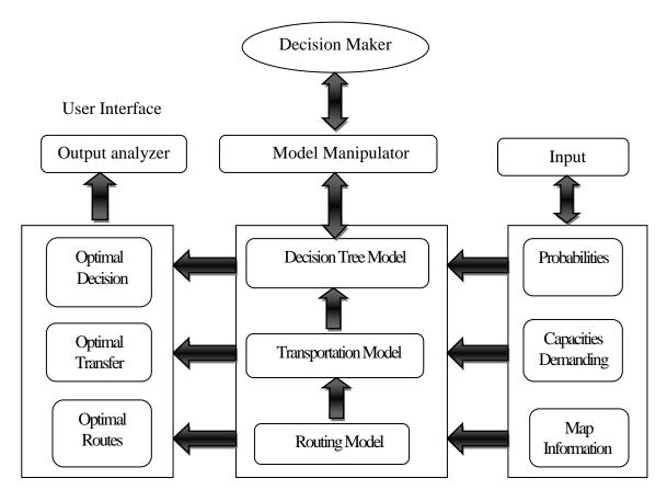
Fig.2.11. Structure of the proposed decision support system (adapted from: Bowen *et al.*, 1989)
