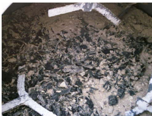
Fig. 2. Rubber particles: (above) as they come after the shredding process; (below) during the mixture of concrete [25].
