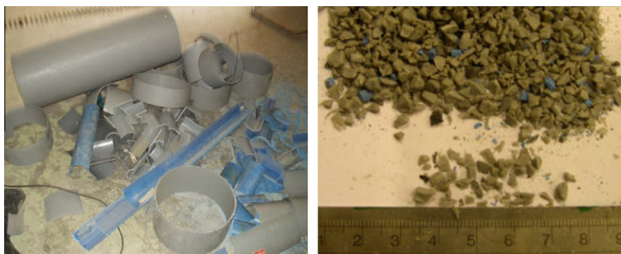
Fig. 14. PVC waste: (left) before crushing; (right) after crushing [95].
