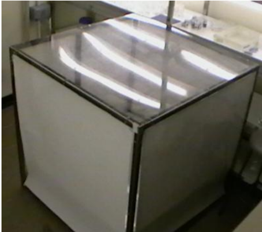
Figure 3.1 Flight Cube used for tethered flight tests of H. axyridis .
