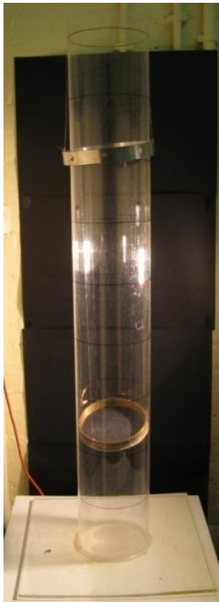
Figure 3-8 Settling tube showing capture net and retrieval collar which was lowered to raise net after each experiment.
